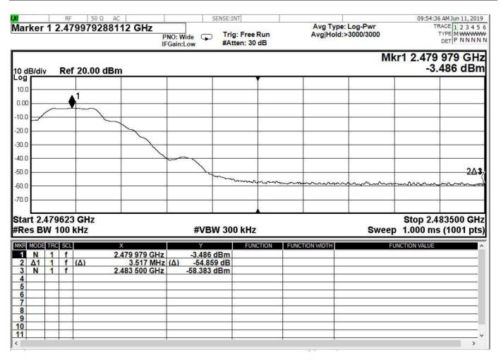
Figure 21 - Band Edge Measurement, High Channel, GFSK
