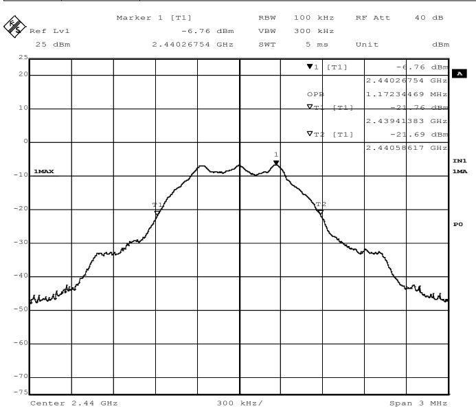
Figure 9 - Occupied Bandwidth, Mid Channel, GMSK
