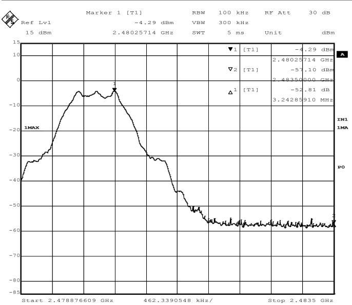
Figure 19 - Band Edge Measurement, High Channel, GMSK
