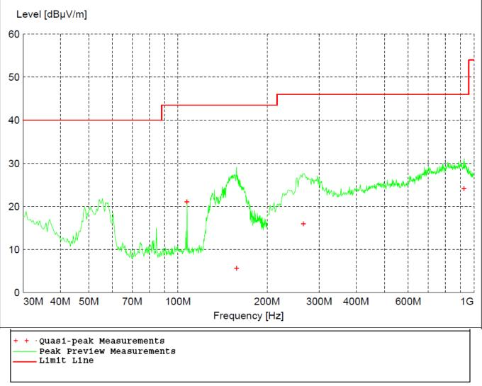
Figure 16 - Radiated Emissions Plot, GMSK
