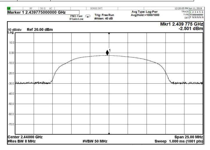
Figure 5 – Output Power, Mid Channel, GFSK
