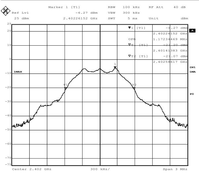
Figure 8 - Occupied Bandwidth, Low Channel, GMSK
