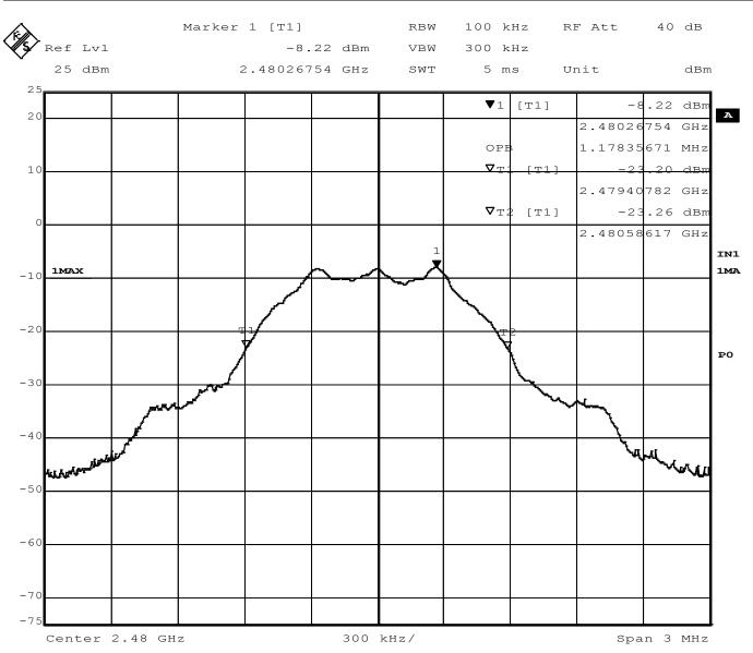
Figure 10 - Occupied Bandwidth, High Channel, GMSK
