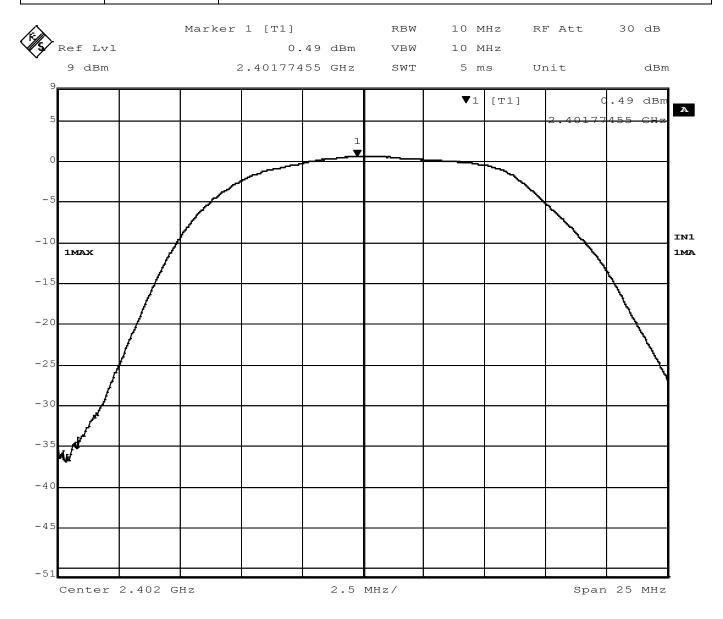
Figure 1 – Output Power, Low Channel, GMSK
