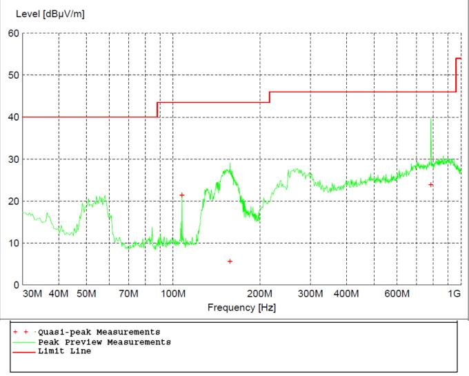
Figure 17 - Radiated Emissions Plot, GFSK
