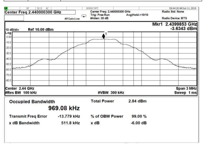
Figure 12 - Occupied Bandwidth, Mid Channel, GFSK
