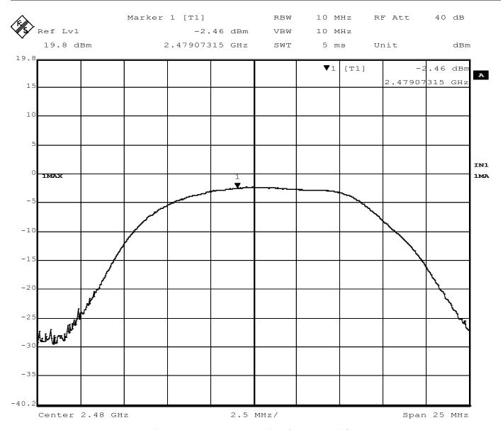
Figure 3 – Output Power, High Channel, GMSK
