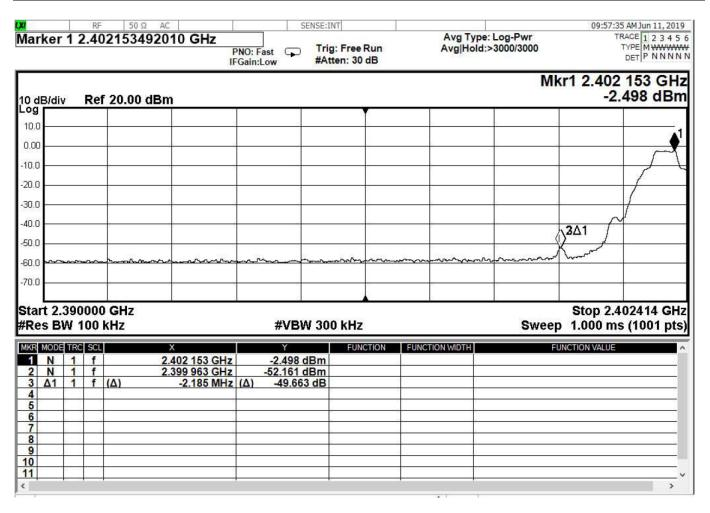
Figure 20 - Band Edge Measurement, Low Channel, GFSK
