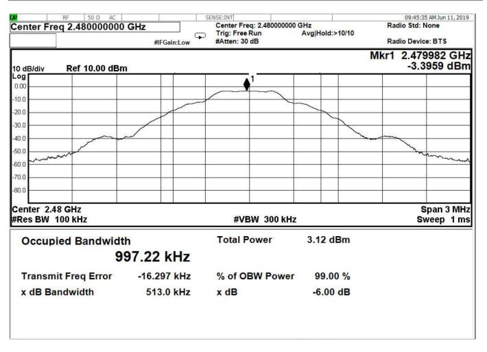
Figure 13 – Occupied Bandwidth, High Channel, GFSK
