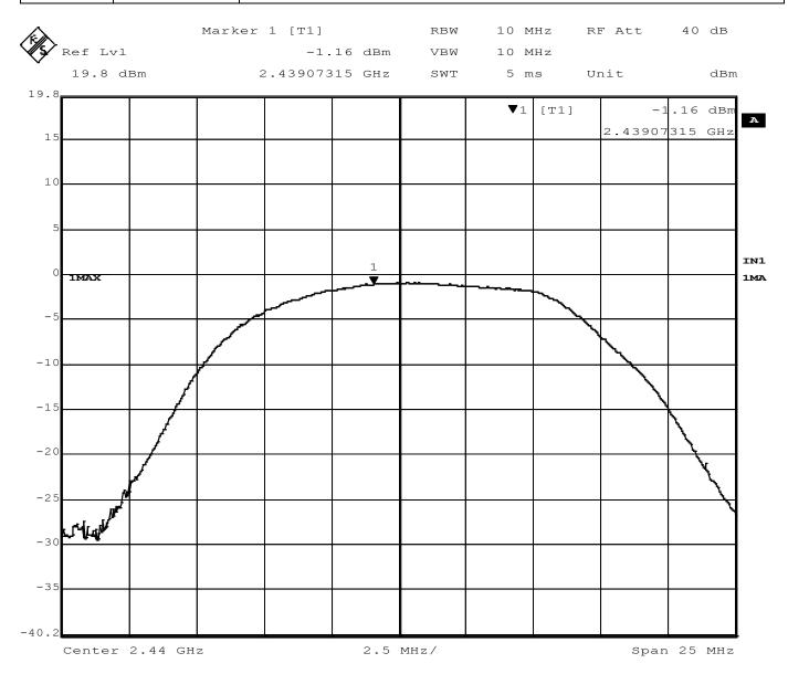
Figure 2 – Output Power, Mid Channel, GMSK
