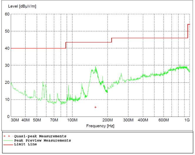
Figure 15 - Radiated Emissions Plot, Receive
