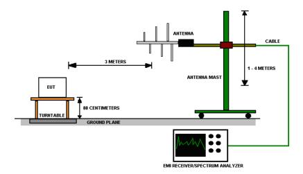
Figure 14 - Radiated Emissions Test Setup
