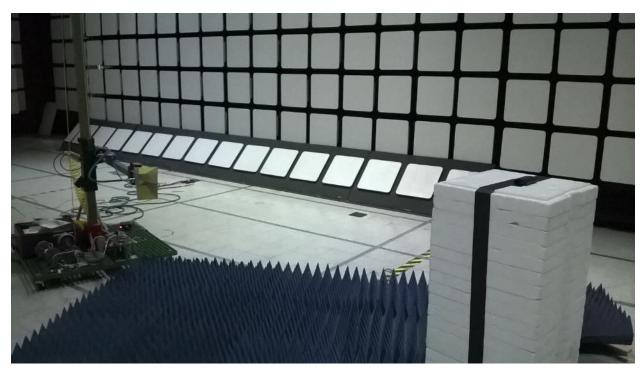
EUT not shown. Photo is intended to show test setup only. 3m, 1-25 GHz
