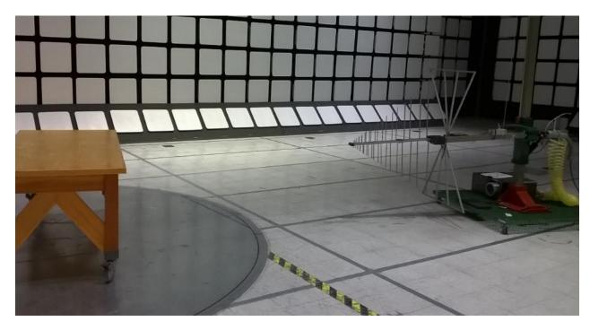
EUT not shown. Photo is intended to show test setup only. 3m, 30 MHz - 1 GHz
