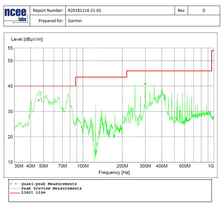
Figure 23 - Radiated Emissions Plot, Low Channel, GMSK, 10 Inch Unit
