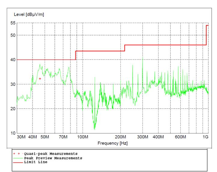
Figure 25 - Radiated Emissions Plot, High Channel, GMSK, 10 Inch Unit
