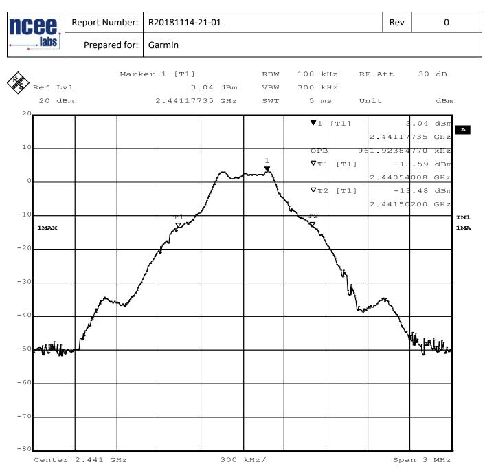
Figure 9 - Occupied Bandwidth, Mid Channel, GFSK
