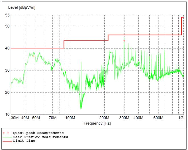
Figure 18 - Radiated Emissions Plot, Mid Channel, GMSK, 12 Inch Unit
