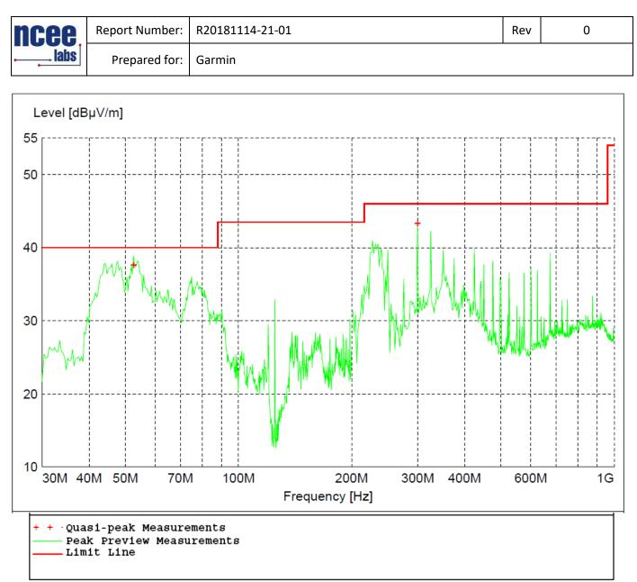
Figure 20 - Radiated Emissions Plot, Low Channel, GFSK, 12 Inch Unit
