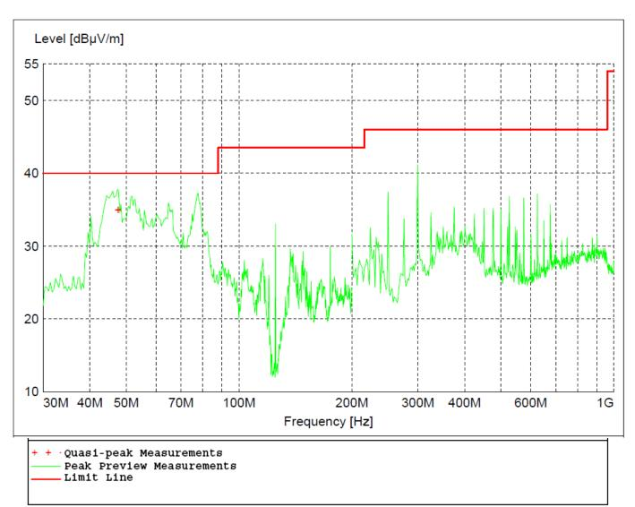
Figure 27 - Radiated Emissions Plot, Mid Channel, GFSK, 10 Inch Unit
