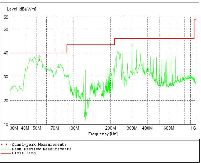
Figure 21 - Radiated Emissions Plot, Mid Channel, GFSK, 12 Inch Unit
