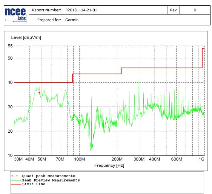
Figure 26 - Radiated Emissions Plot, Low Channel, GFSK, 10 Inch Unit
