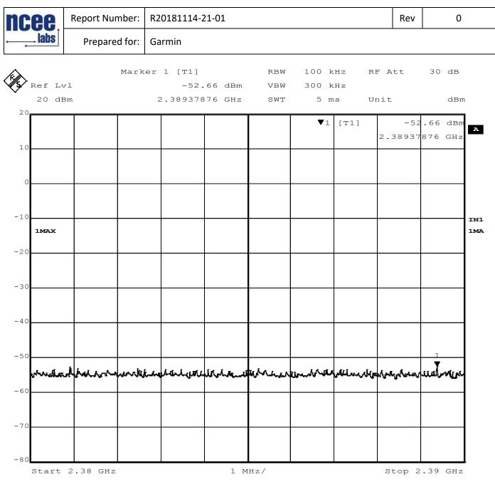
Figure 35 –Band Edge, Low Channel, Restricted, GMSK
