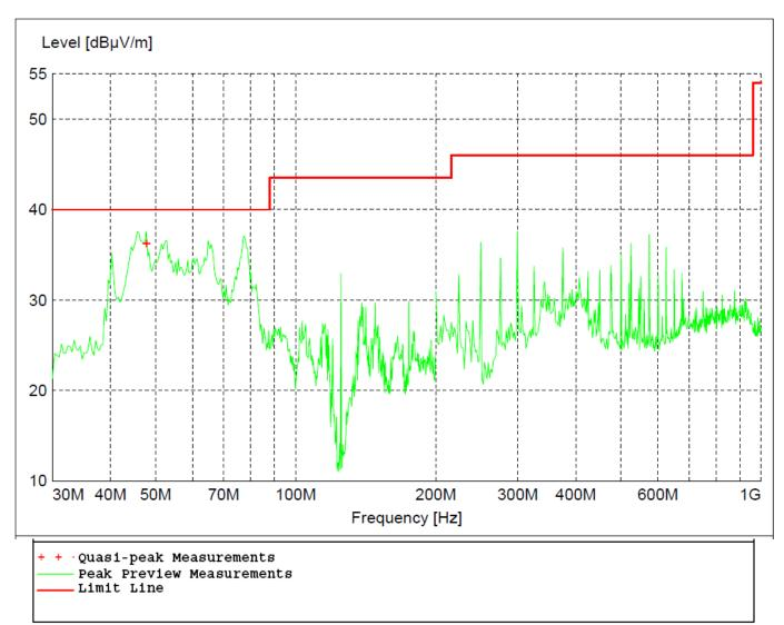
Figure 24 - Radiated Emissions Plot, Mid Channel, GMSK, 10 Inch Unit
