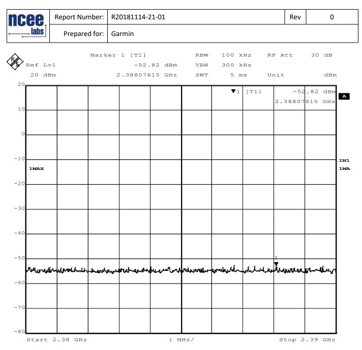
Figure 33 - Band Edge, Low Channel, Restricted, GFSK
