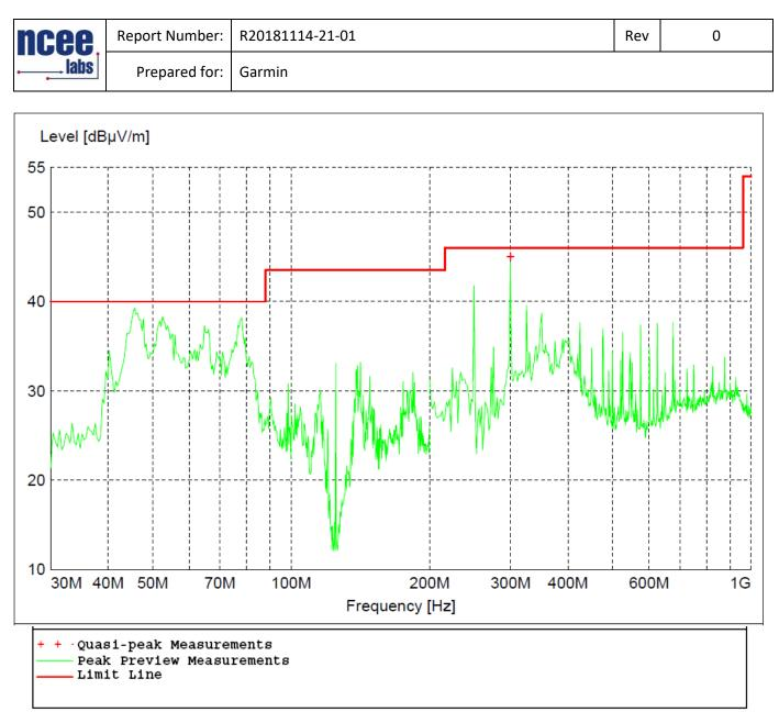
Figure 16 - Radiated Emissions Plot, Receive, 10 Inch Unit
