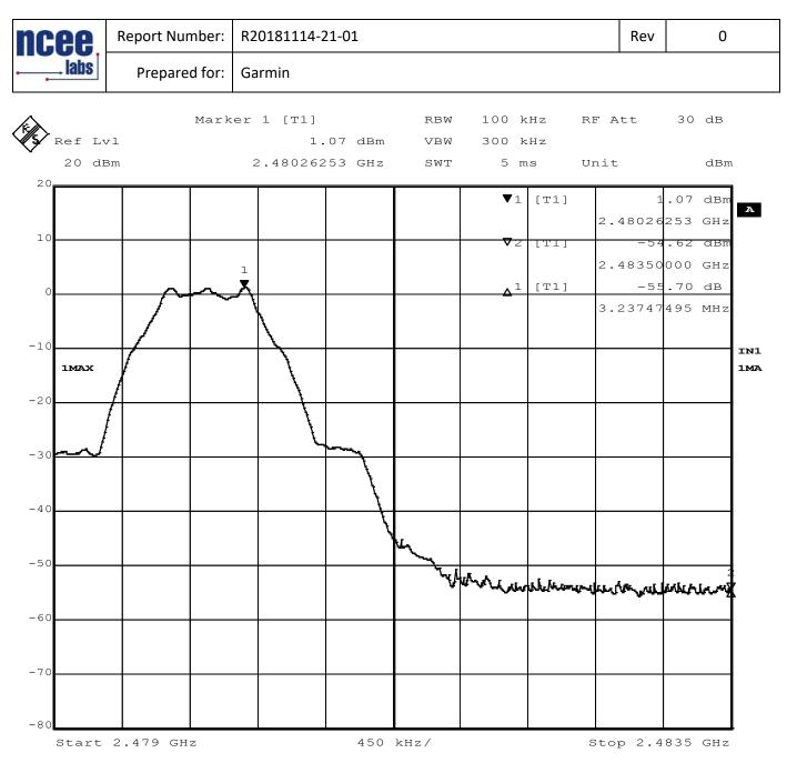
Figure 32 – Band Edge Measurement, High Channel, Unrestricted, GMSK
