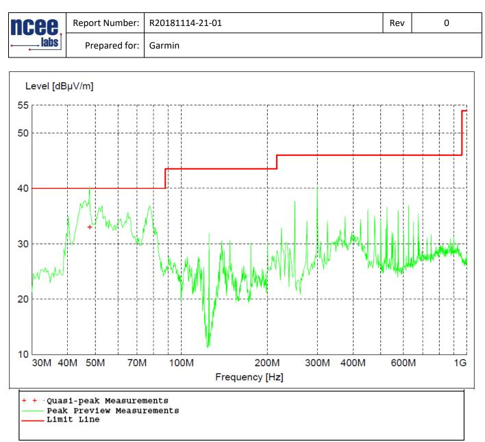
Figure 28 - Radiated Emissions Plot, High Channel, GFSK, 10 Inch Unit
