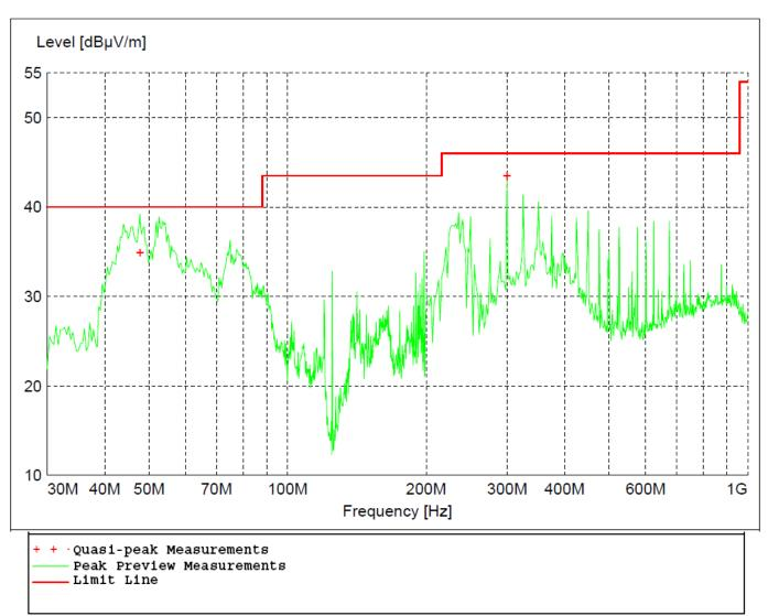
Figure 19 - Radiated Emissions Plot, High Channel, GMSK, 12 Inch Unit
