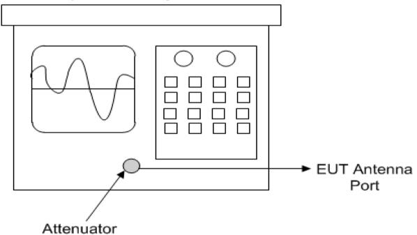
Diagram 4 Test arrangement for Antenna Port Conducted emissions
