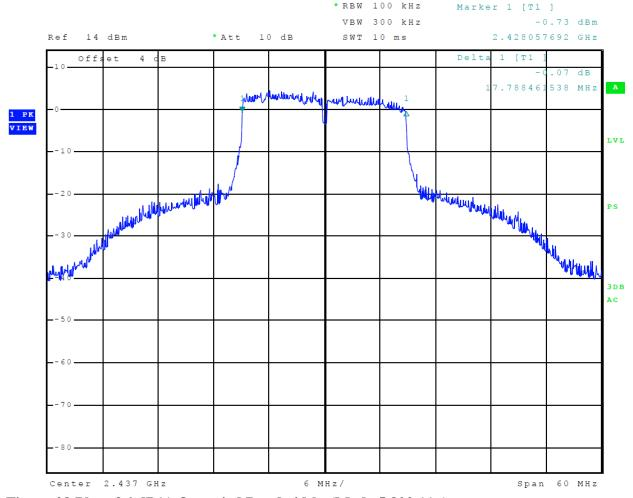
Figure 28 Plot of 6-dB% Occupied Bandwidth (Mode 5 802.11n)
