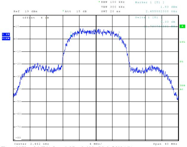
Figure 24 Plot of 6-dB% Occupied Bandwidth (Mode 5 802.11b)
