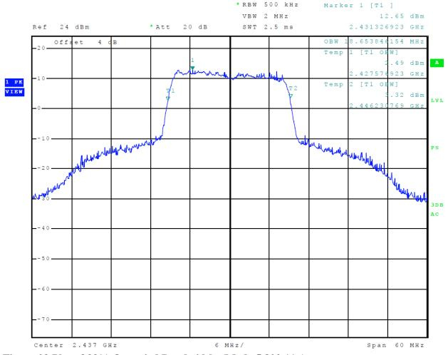
Figure 29 Plot of 99% Occupied Bandwidth (Mode 5 802.11n)
