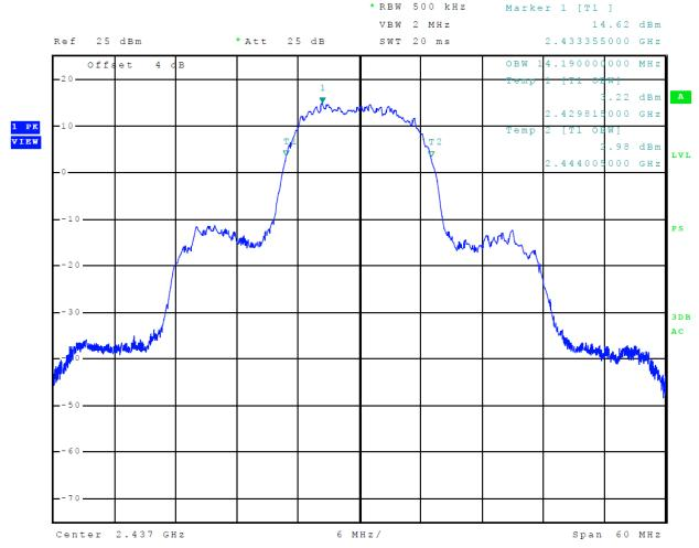
Figure 25 Plot of 99% Occupied Bandwidth (Mode 5 802.11b)
