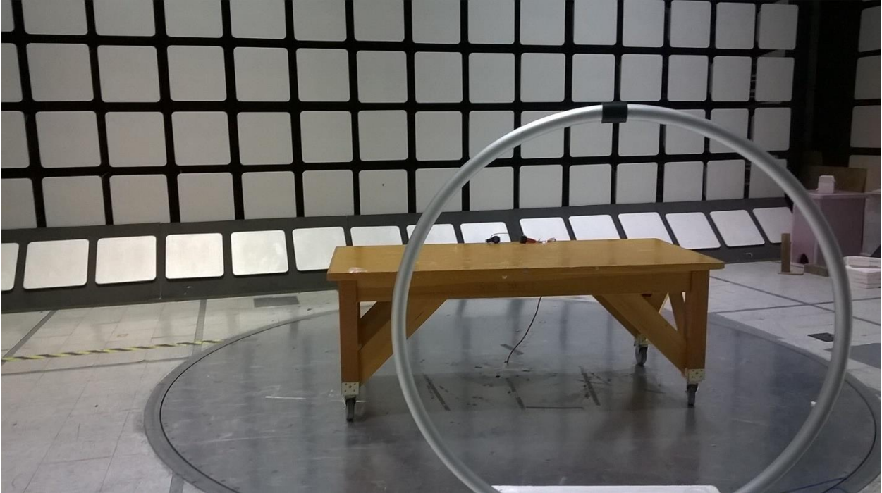
Figure 3 - Radiated emissions test setup, 10 MHz - 30 MHz
