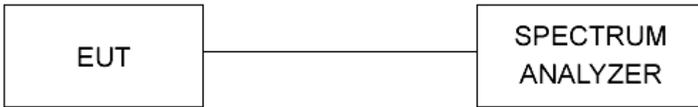
Figure 7 - Bandwidth Measurements Test Setup
