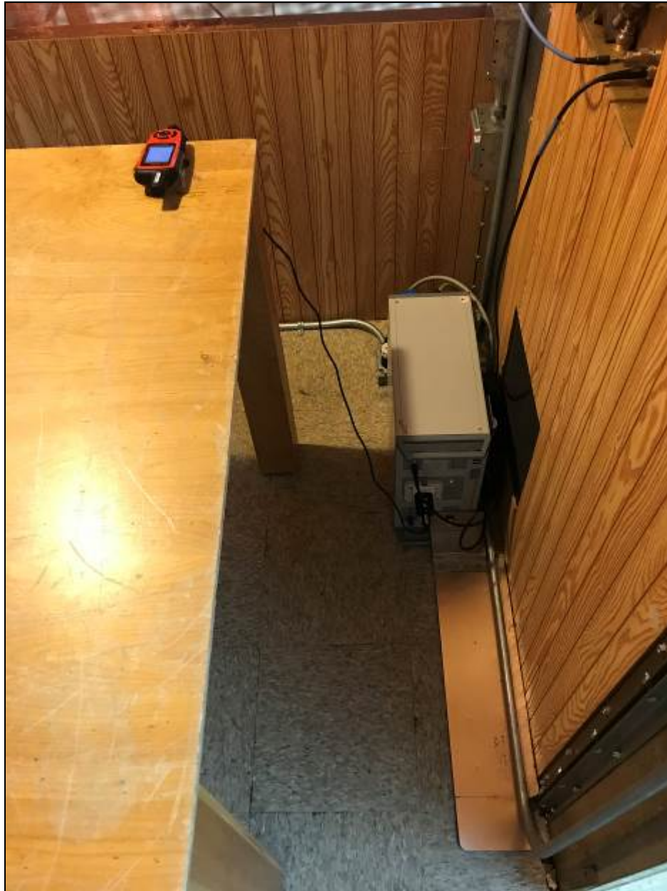
Photograph 3: AC Conducted Emissions Testing – AC Adapter ADP-5BW B C.C:A
