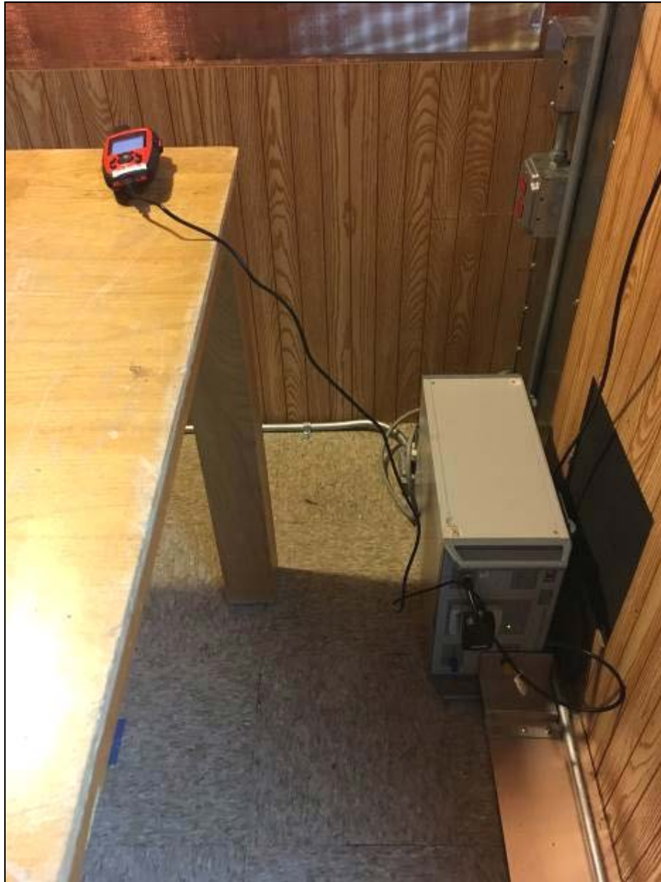
Photograph 5: AC Conducted Emissions Testing – AC Adapter PSAI05R-050Q
