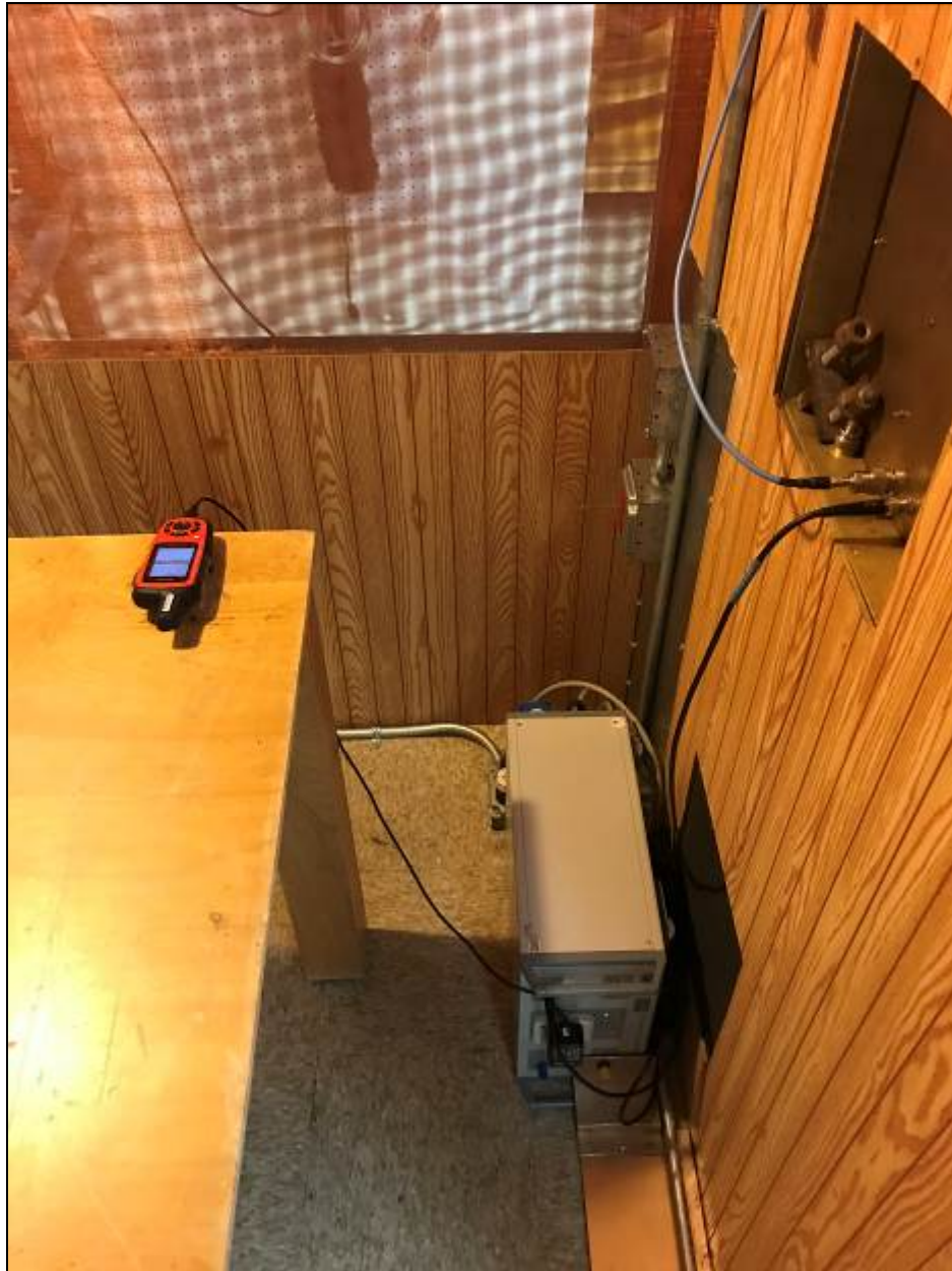
Photograph 4: AC Conducted Emissions Testing – AC Adapter PSAF10R-050Q
