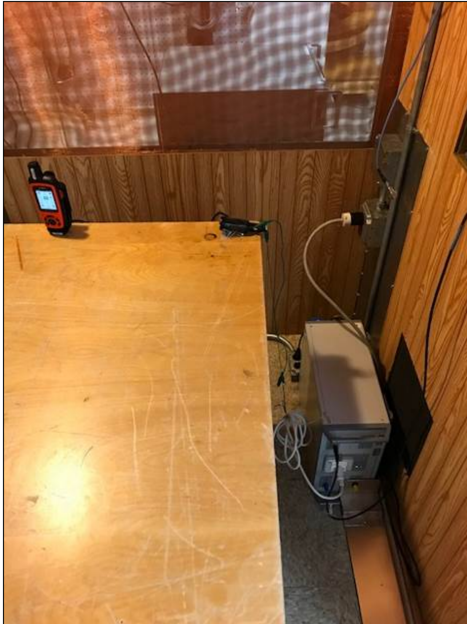
Photograph 6: DC Conducted Emissions Testing – Car Charger Adapter RF-279-G021-0
