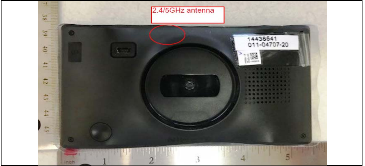
Figure A03504 – Antenna Location D5
