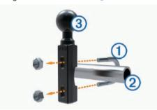
**2** Tighten the nuts to secure the base.
