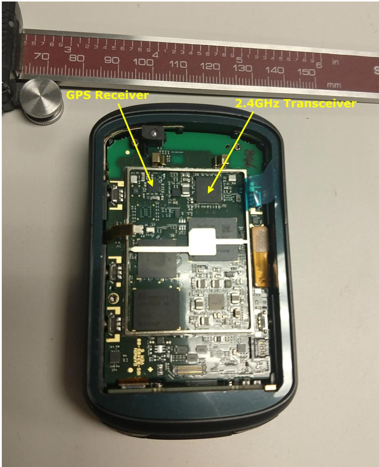
Top side of PCB with cover of shielded enclosure removed to show transceivers.
