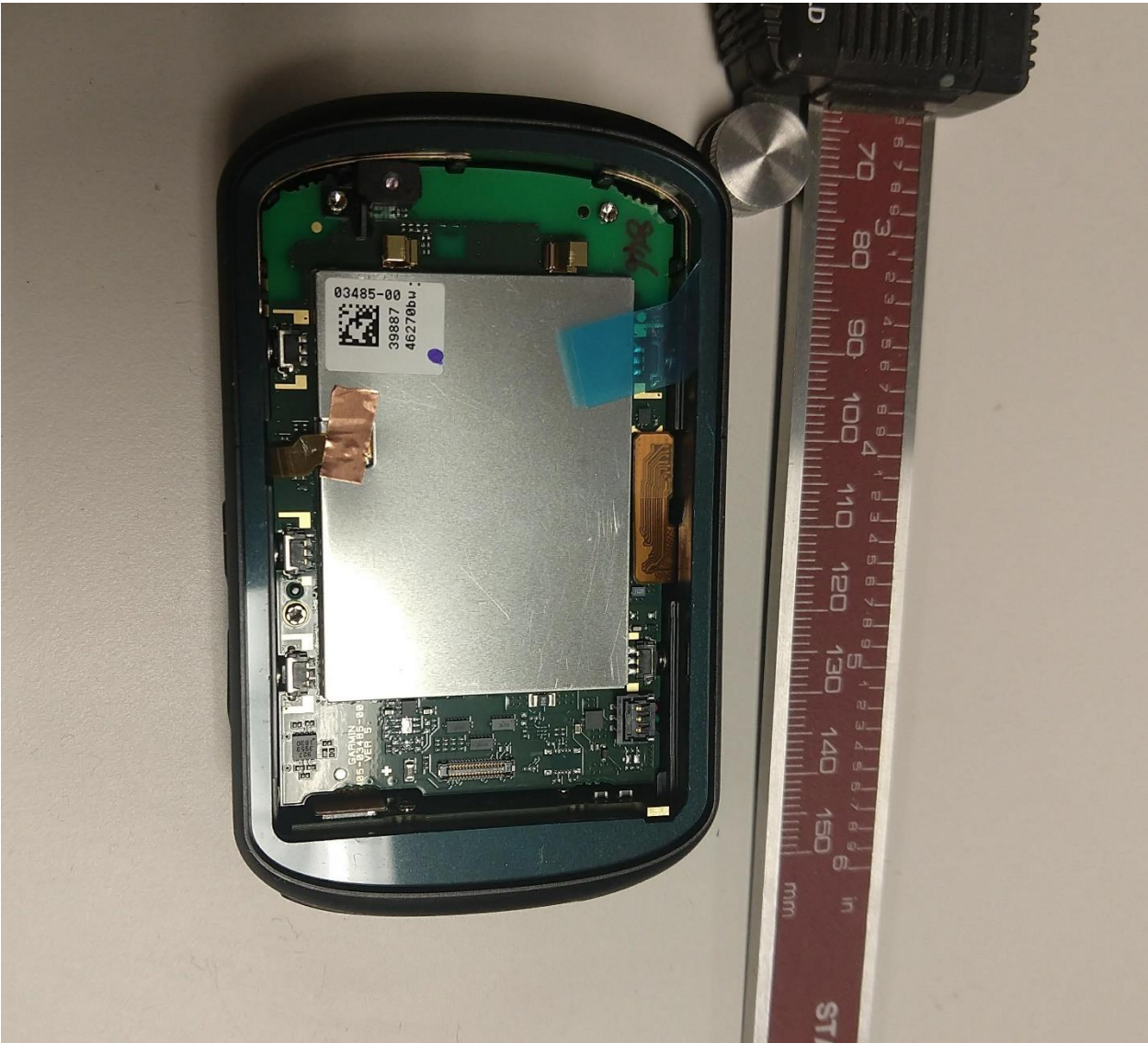
Top of PCB with cover on shielded enclosure.
