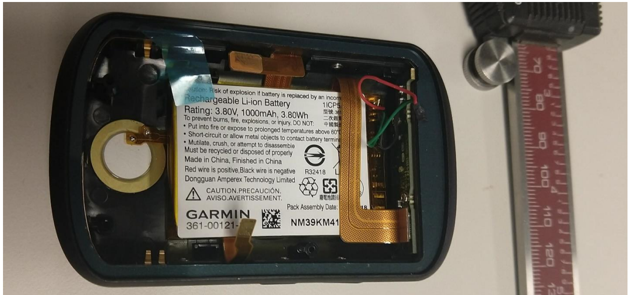
PCB removed to show battery.
