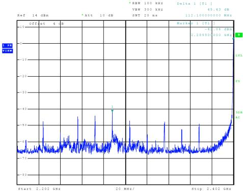
Figure 3 Plot of Transmitter Emissions (Low Band Edge)
