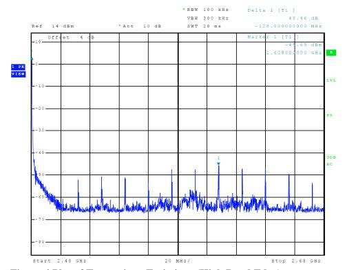
Figure 4 Plot of Transmitter Emissions (High Band Edge)
