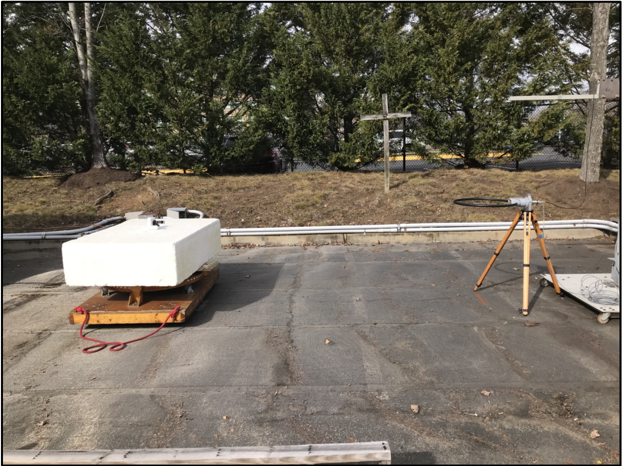
Photograph 2: Radiated Emissions Testing – Side View (Below 30 MHz)
