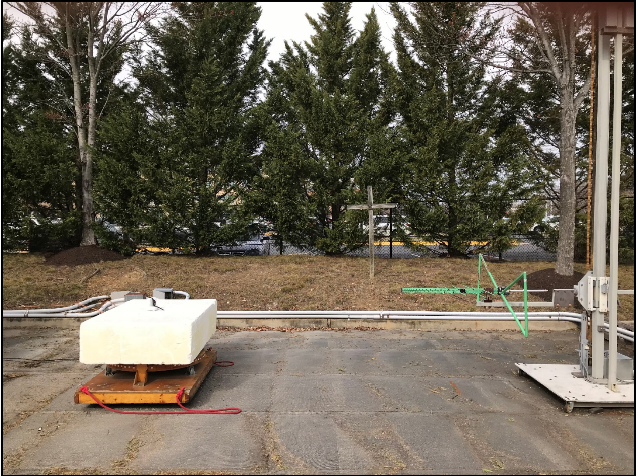
Photograph 1: Radiated Emissions Testing – Side View (Above 30 MHz, below 1 GHz)
