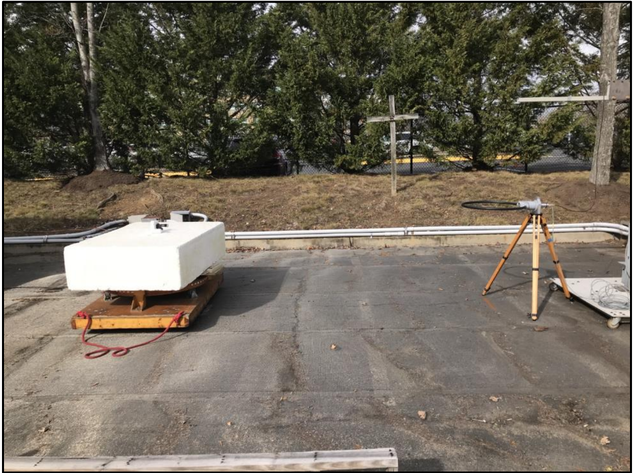
Photograph 2: Radiated Emissions Testing – Side View (Below 30 MHz)
