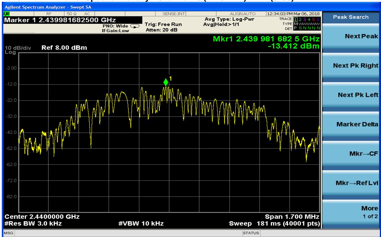
Plot 8-11: Power Spectral Density: Channel 19 (2440 MHz): BLE (0x55)
