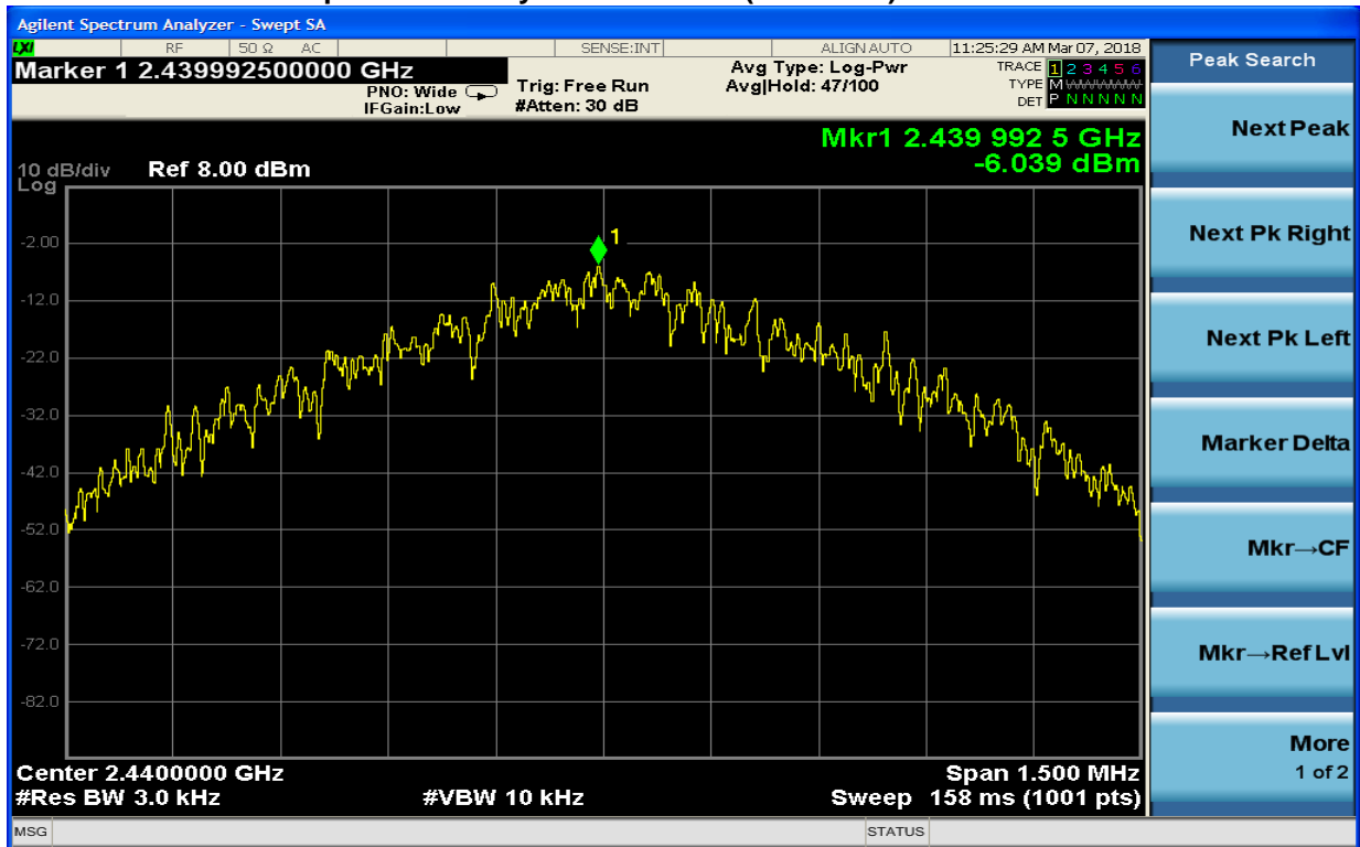
Plot 8-2: Power Spectral Density: Channel Mid (2441 MHz): ANT+
