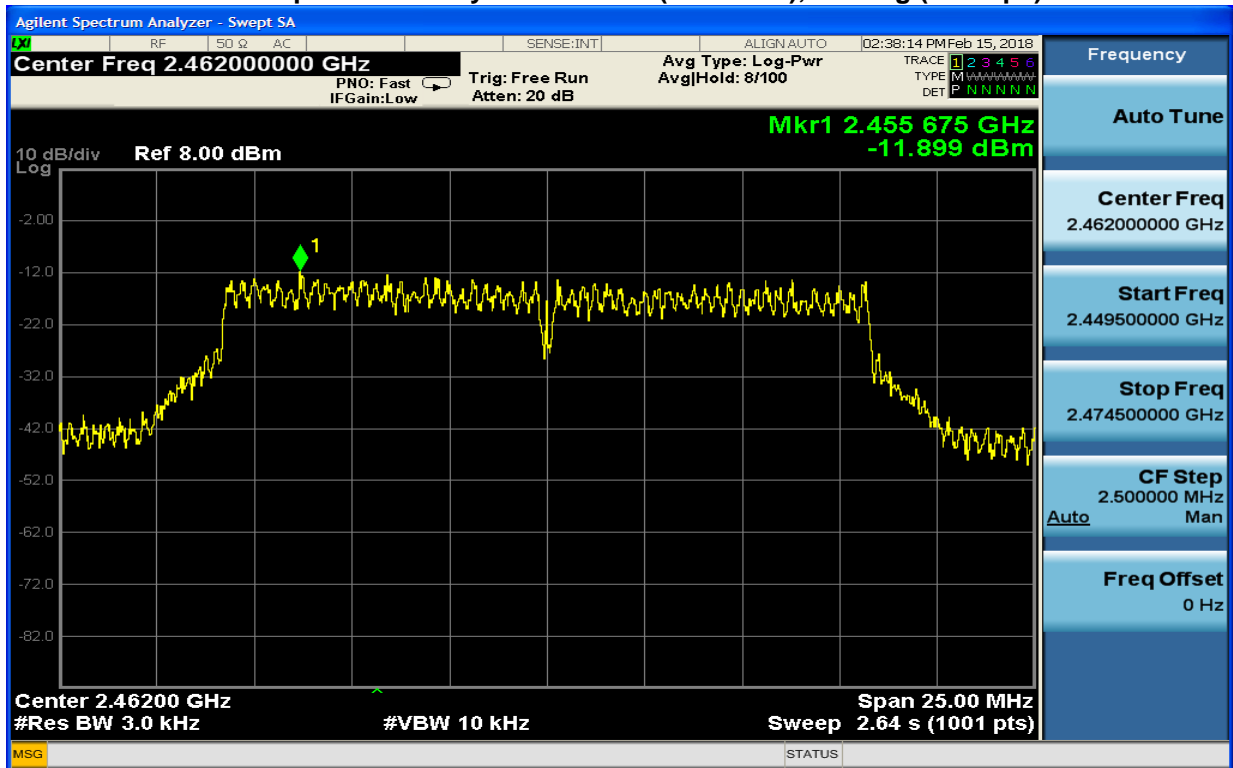
Plot 8-18: Power Spectral Density: Channel 11 (2462 MHz); 802.11g (54 Mbps)
