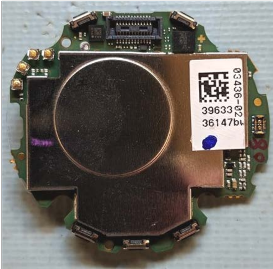
Main Board with Shield – Top View
