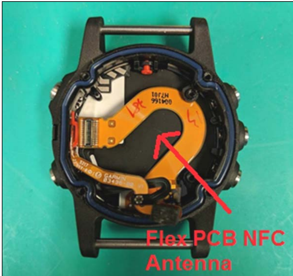
Display Assembly with NFC Antenna
