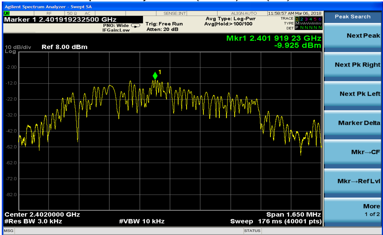
Plot 8-10: Power Spectral Density: Channel 0 (2402 MHz) – BLE (0x55)
