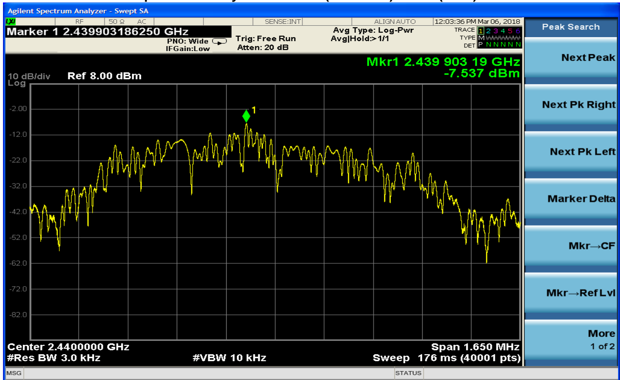
Plot 8-8: Power Spectral Density: Channel 19 (2440 MHz) – BLE (0x0F)
