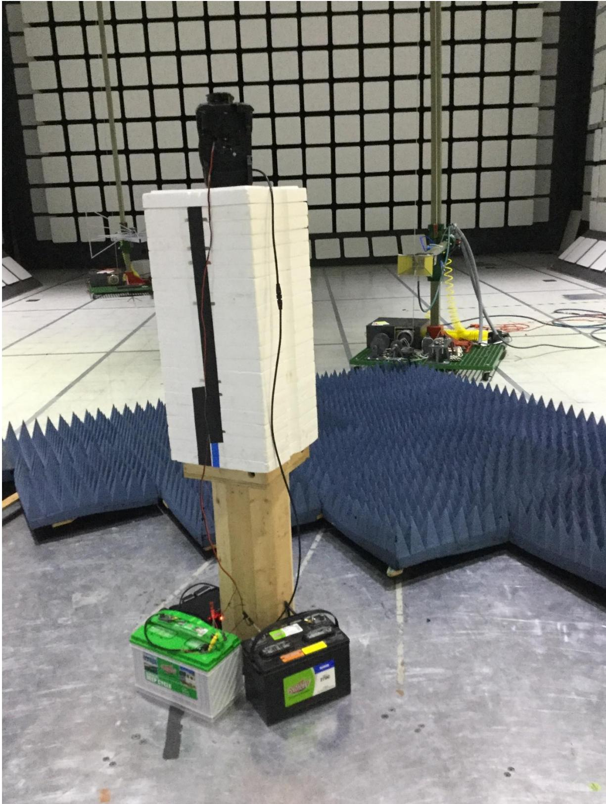
Radiated emissions test, 1GHz – 25GHz
