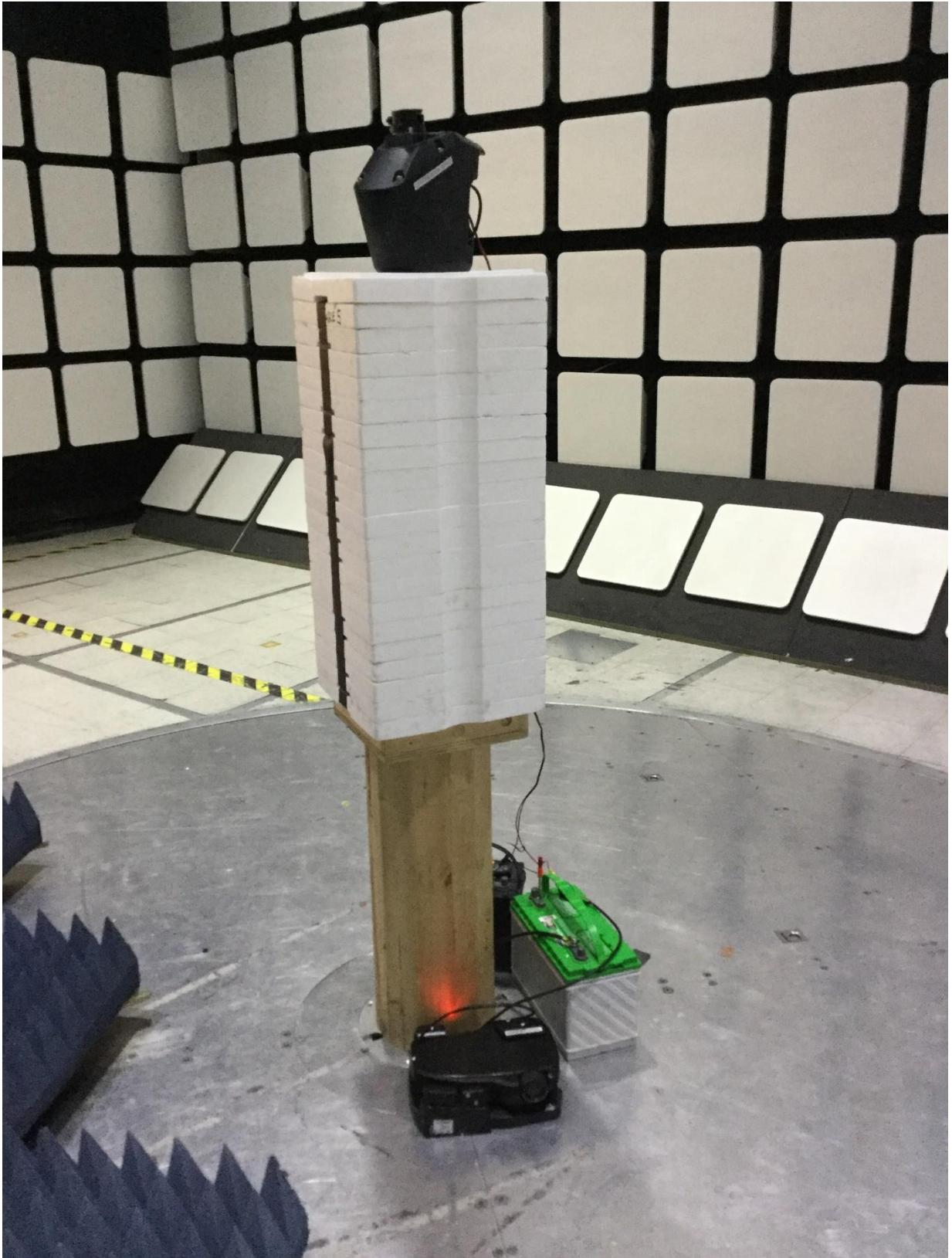
Radiated emissions test, 1GHz – 25GHz
