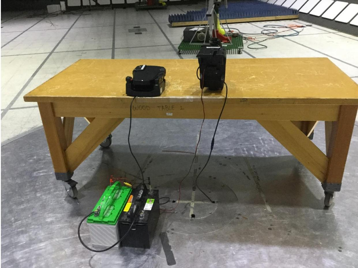
Radiated emissions test, 30MHz – 1GHz
