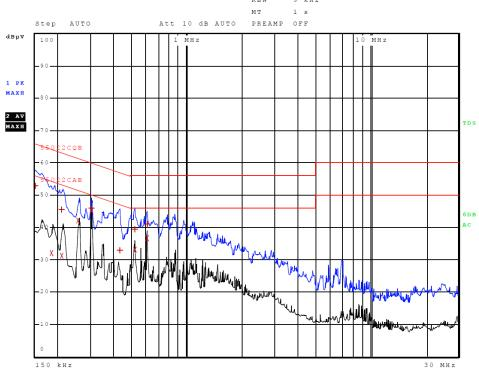
Figure 5 AC Line Conducted emissions of EUT line 1 (#4, EUT – Computer)
