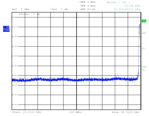
Figure 13 Plot of Transmitter Emissions (Low Band Edge, 25 MHz Chnl, 24 GHz)
