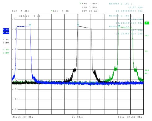
Figure 11 Plot of Transmitter Emissions (In 24.0-24.25 GHz Band, 25 MHz Chnl, 24 GHz)
