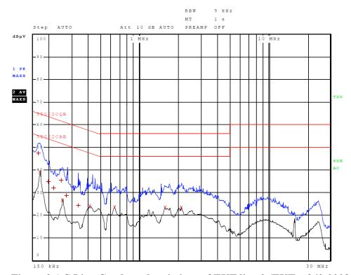
Figure 2 AC Line Conducted emissions of EUT line 2 (EUT – 362-00086-01)
