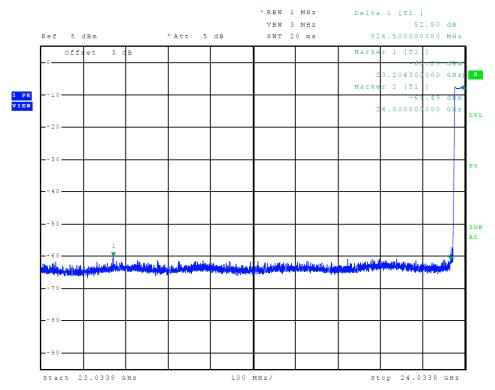
Figure 17 Plot of Transmitter Emissions (Low Band Edge, 50 MHz Chnl, 24 GHz)
