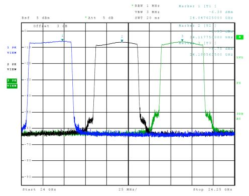
Figure 15 Plot of Transmitter Emissions (In 24.0-24.25 GHz Band, 50 MHz Chnl, 24 GHz)
