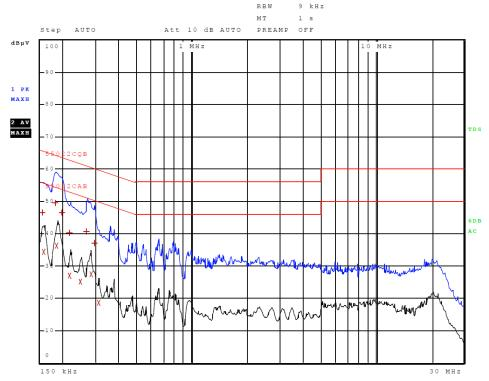
Figure 3 AC Line Conducted emissions of EUT line 1 (EUT – 362-00087-00)
