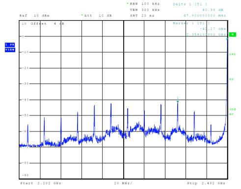
Figure 9 Plot of Transmitter Emissions (Low Band Edge, 2400 MHz Band)
