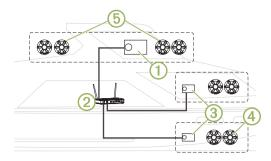
In the image above, a Apollo RA770 stereo ① connects to a wireless router ② and to two Apollo SRX400 zone stereos ③. You can connect a FUSION PartyBus zone stereo to a single speaker zone ④. You can connect a FUSION PartyBus stereo to multiple speaker zones ⑤ to cover a larger area.
