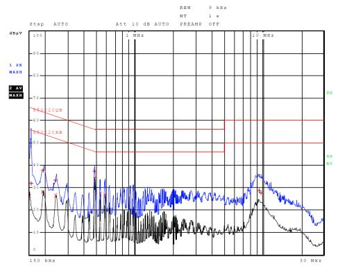
Figure 2 AC Line Conducted emissions of EUT line 2 (#2, EUT – 362-00091-00)
