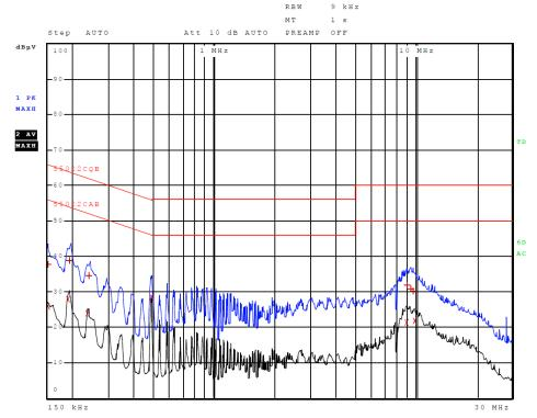
Figure 1 AC Line Conducted emissions of EUT line 1 (#2, EUT – 362-00091-00)
