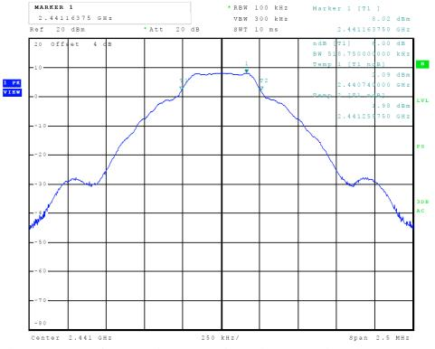
Figure 27 Plot of Transmitter 6-dB Occupied Bandwidth (BLE-Mode 3)
