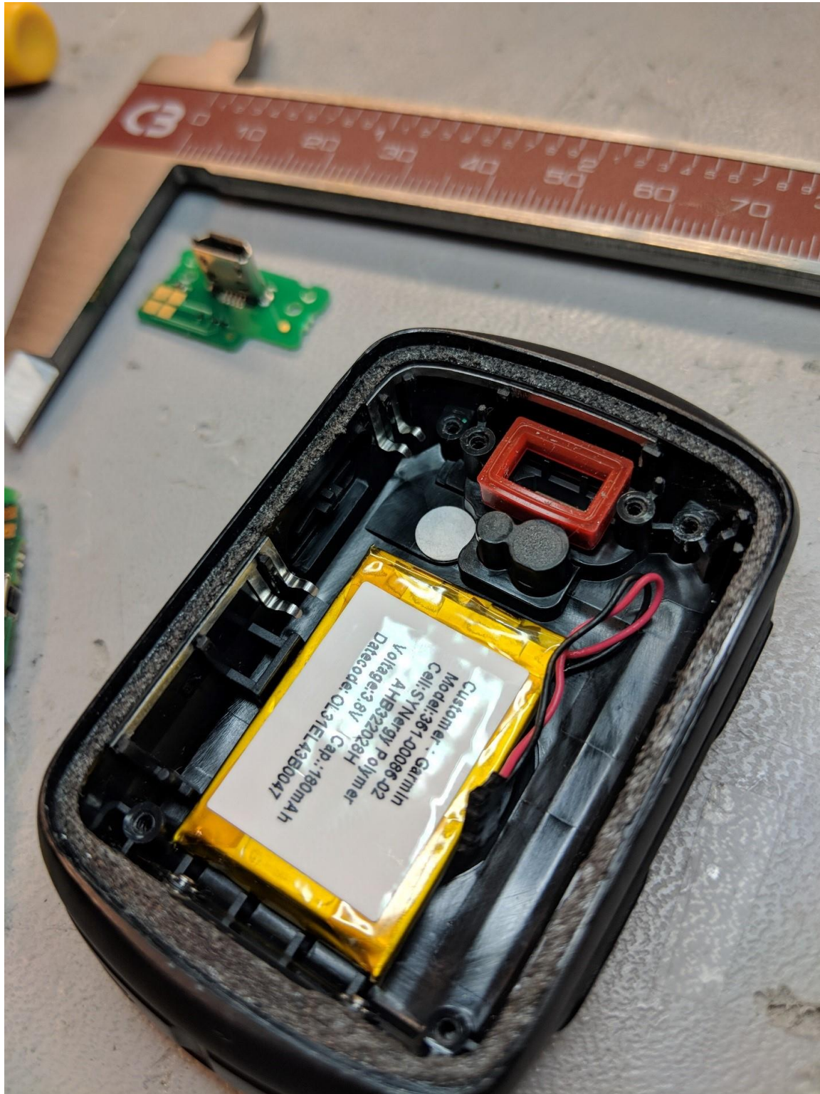
Main PCB removed showing battery
