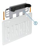
NOTE: It is recommended to install the camera above the license plate, if possible. If there is not enough room above the license plate on your vehicle, you can configure the mount for installation below the license plate (page 2).
