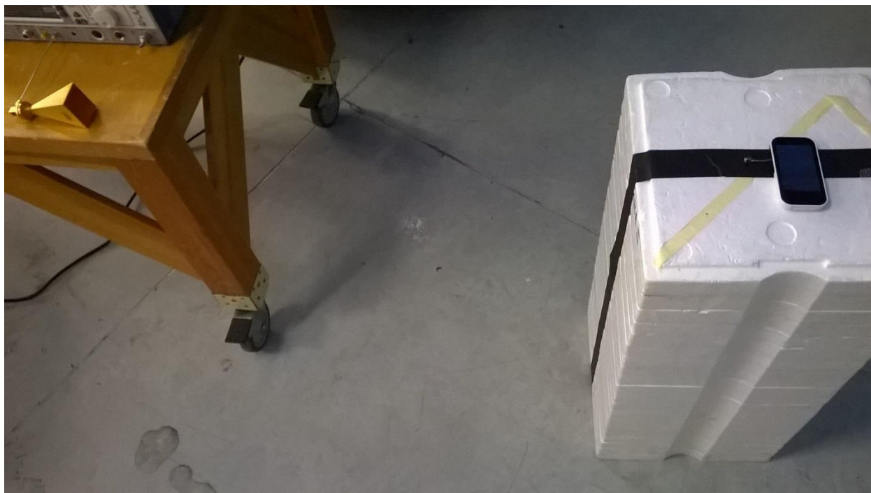
Figure 7 – Radiated Emissions Test Setup, 40 – 50 GHz
