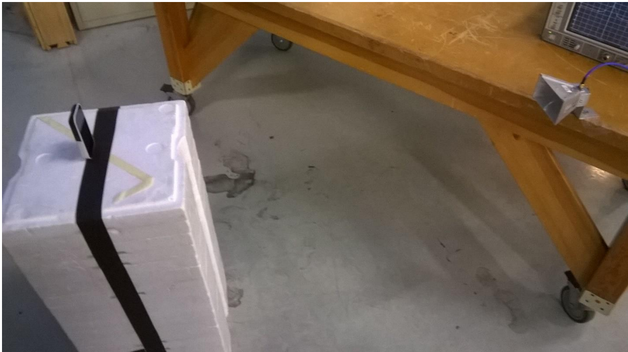
Figure 6 - Radiated Emissions Test Setup, 26.5 – 40 GHz
