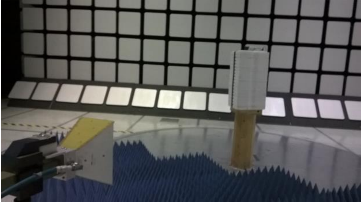
Figure 1 - Radiated Emissions Test Setup, 1 - 25 GHz
