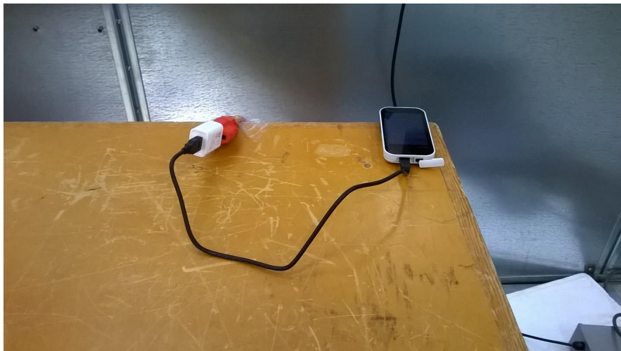
Figure 9 – Conducted Emissions Test Setup
