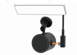
3 Route the power cable to your vehicle power outlet. The included long, lightweight power cable is designed to be routed out of sight. To hide the cable, you can route it around the windshield and tuck it into the gap between the windshield and the trim.
