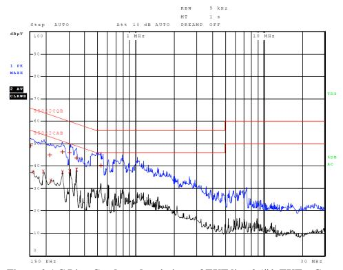
Figure 2 AC Line Conducted emissions of EUT line 2 (#4, EUT – Computer)
