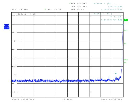
Figure 12 Plot of Transmitter Emissions (Low Band Edge, BT GFSK)
