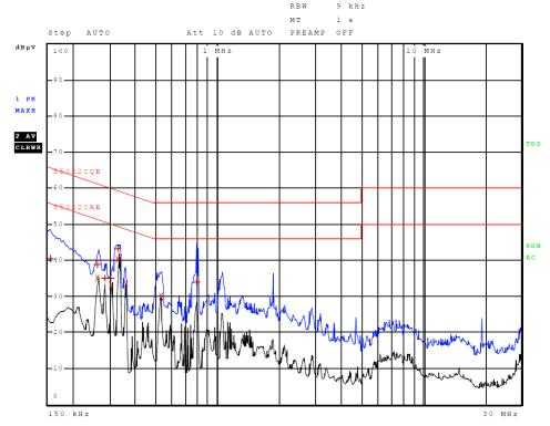
Figure 1 AC Line Conducted emissions of EUT line 1 (#4, EUT – Computer)
