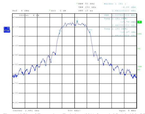
Figure 10 Plot of Transmitter Emissions (99% Occupied Bandwidth, BT 8DPSK)
