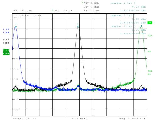
Figure 5 Plot of Transmitter Emissions (Operation in 2402-2480 MHz, BT 4PI-DQPSK)
