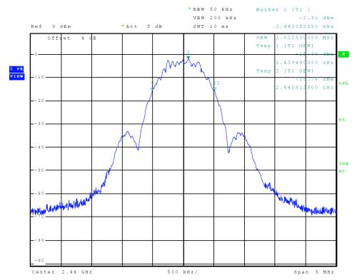
Figure 7 Plot of Transmitter Emissions (99% Occupied Bandwidth, BLE)
