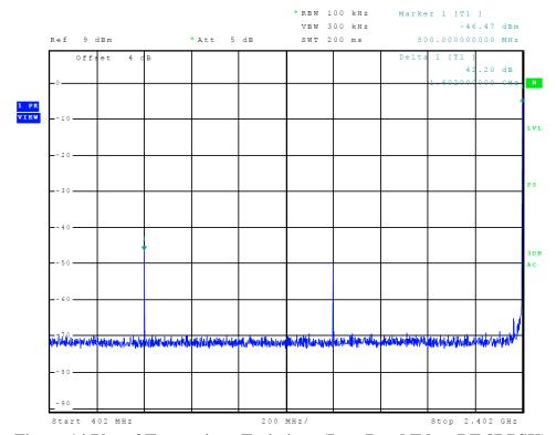
Figure 14 Plot of Transmitter Emissions (Low Band Edge, BT 8DPSK)
