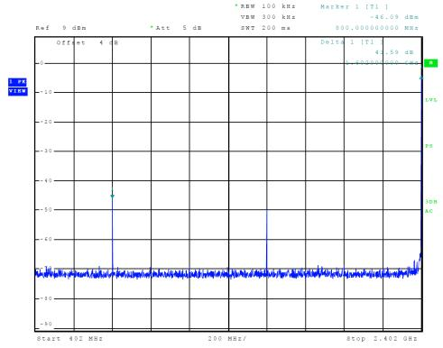
Figure 13 Plot of Transmitter Emissions (Low Band Edge, BT 4PI-DQPSK)
