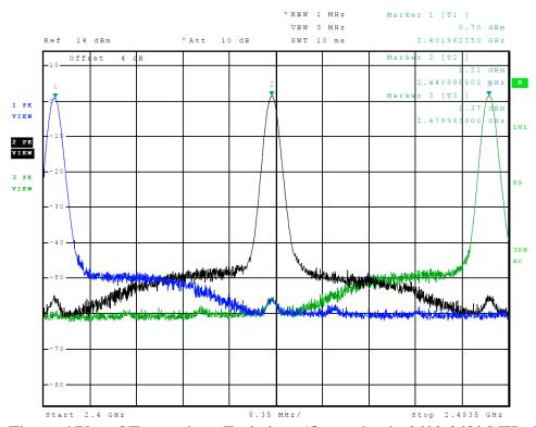
Figure 6 Plot of Transmitter Emissions (Operation in 2402-2480 MHz, BT 8DPSK)
