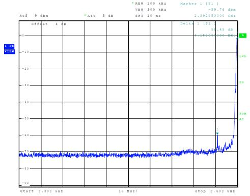
Figure 11 Plot of Transmitter Emissions (Low Band Edge, BLE)
