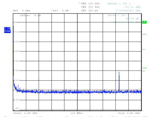
Figure 18 Plot of Transmitter Emissions (High Band Edge, BT 8DPSK)
