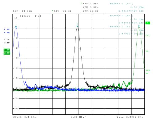
Figure 4 Plot of Transmitter Emissions (Operation in 2402-2480 MHz, BT GFSK)
