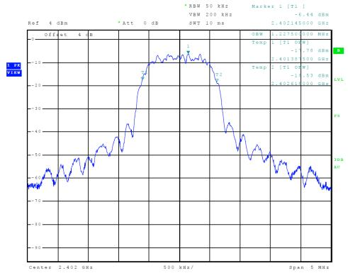
Figure 9 Plot of Transmitter Emissions (99% Occupied Bandwidth, BT 4PI-DQPSK)
