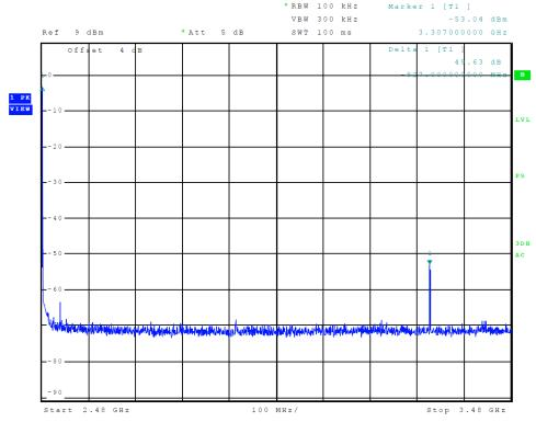
Figure 17 Plot of Transmitter Emissions (High Band Edge, BT 4PI-DQPSK)
