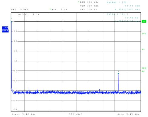
Figure 15 Plot of Transmitter Emissions (High Band Edge, BLE)
