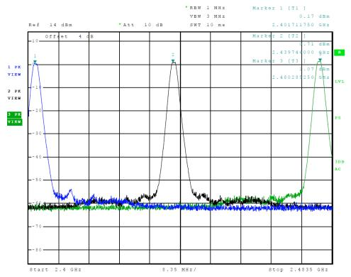
Figure 3 Plot of Transmitter Emissions (Operation in 2402-2480 MHz, BLE)
