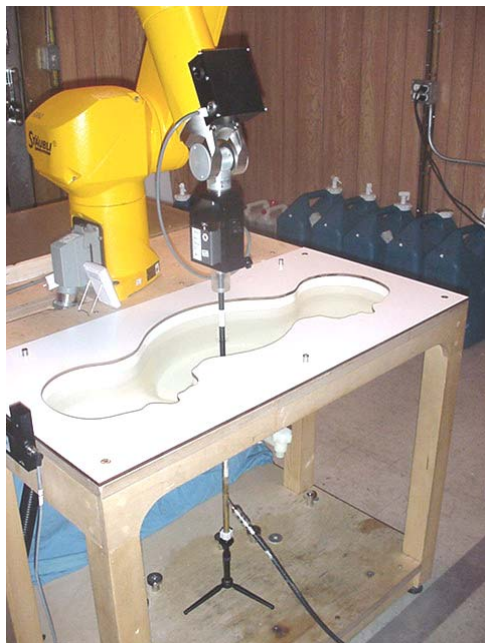
DASY 4 SAR System with SAM Phantom
