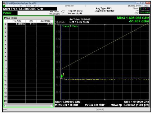
Figure 12 – Part 25.216(g), Transmitting at 1620.979167 MHz, Conducted Measurement \*Limits have been converted from dBW to dBm. dBW = dBm + 30
