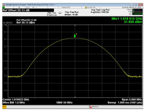
Figure 24 – Radiated Average Power Measurement, Iridium, Low Reference offset includes EIRP conversion and corrections
