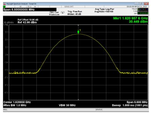
Figure 3 – Conducted Average Output Power, Transmitting at 1620.979167 MHz
