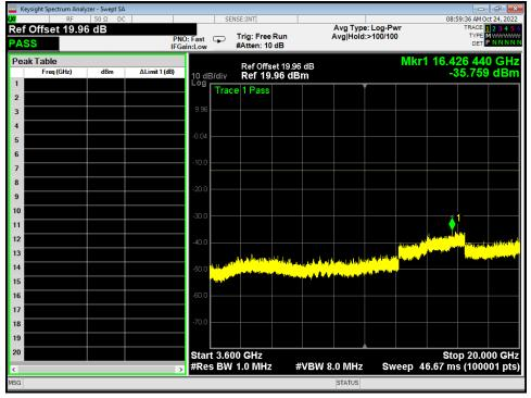
Figure 16 – Conducted Spurious Plot, 3.6G – 20G
