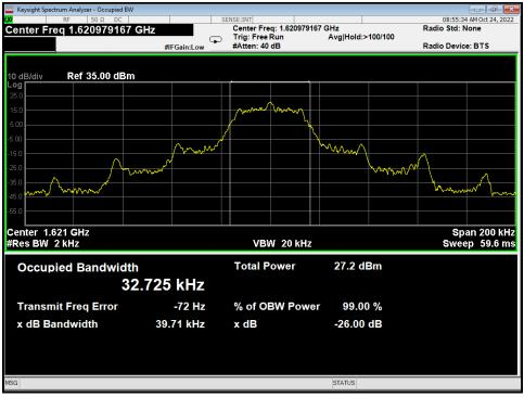
Figure 18 – Supporting Plots for modulation characteristic, Mid Channel
