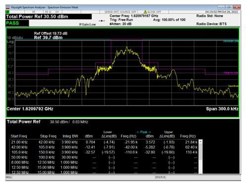
Figure 6 – Part 25.202(f) Mask, Transmitting at 1620.979167 MHz
