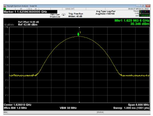
Figure 4 – Conducted Average Output Power, Transmitting at 1625.979167 MHz
