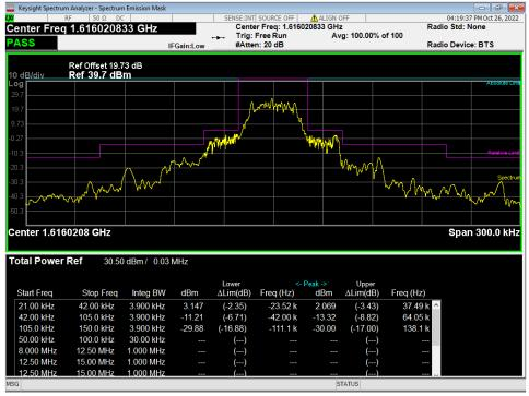
Figure 5 – Part 25.202(f) Mask, Transmitting at 1616.020833 MHz
