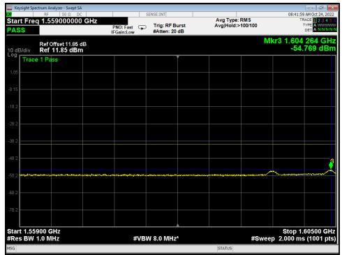
Figure 9 – Part 25.216(c), Transmitting at 1620.979167 MHz, Conducted Measurement \*Limits have been converted from dBW to dBm. dBW = dBm + 30 Antenna Gain = 1.396 dB; Limit = -40.00 dBm; Margin=-40.00-(-54.769+1.396) =16.17 dB
