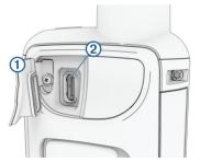
2 Plug the small end of the power cable into the charging port ② on the device.
