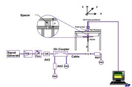
**Figure 7.1 Dipole Verification Test Setup**
