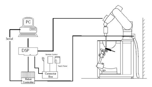
Figure 2.1 SAR Measurement System Setup
