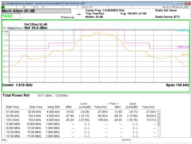
Figure 2 – Part 25.202(f) Mask, Transmitting at 1616.028330 MHz
