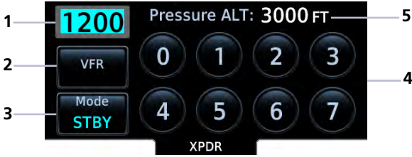
XPDR Control Panel
