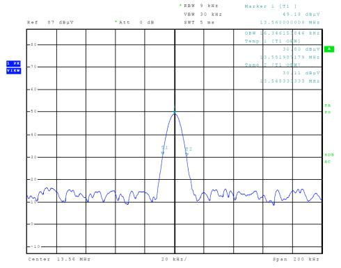
Figure 9 Plot of NFC 99 percent Occupied Bandwidth
