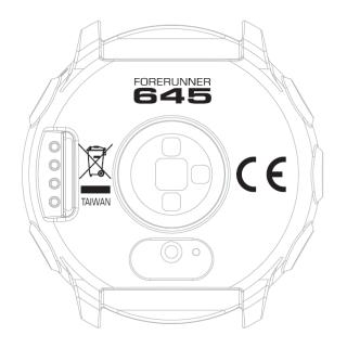
PMN is permanently affixed to the back of the unit via laser etching as shown above.
