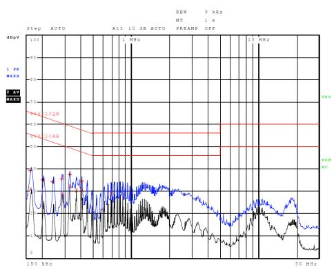
Figure 4 AC Line Conducted emissions of EUT line 2 (#3, EUT – 320-0008-201)
