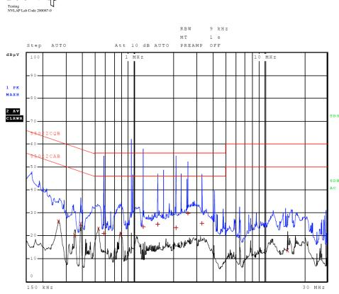
Figure 1 AC Line Conducted emissions of EUT line 1 (#2, EUT – Computer)
