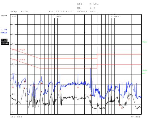
Figure 2 AC Line Conducted emissions of EUT line 2 (#2, EUT – Computer)
