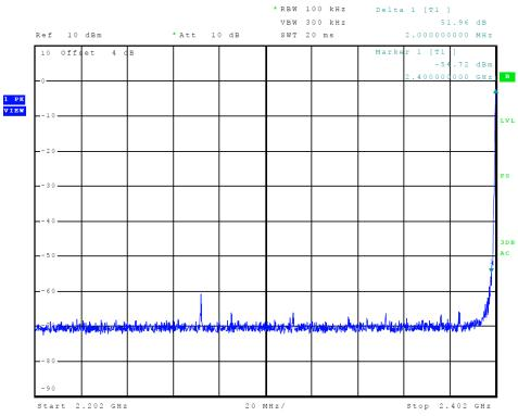
Figure 13 Plot of Transmitter Emissions (Low Band Edge, BLE)
