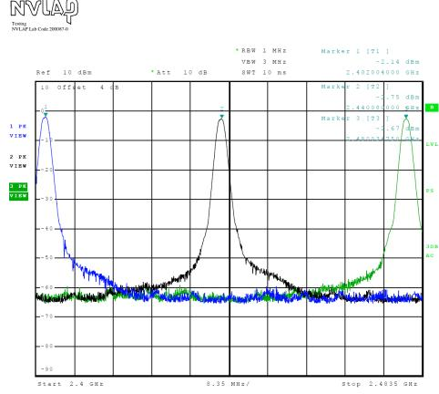
Figure 11 Plot of Transmitter Emissions (Operation in 2402-2480 MHz, BLE)
