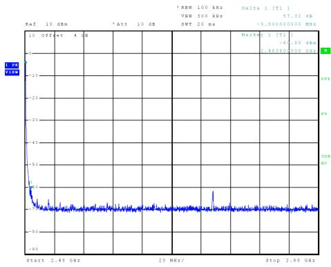
Figure 14 Plot of Transmitter Emissions (High Band Edge, BLE)
