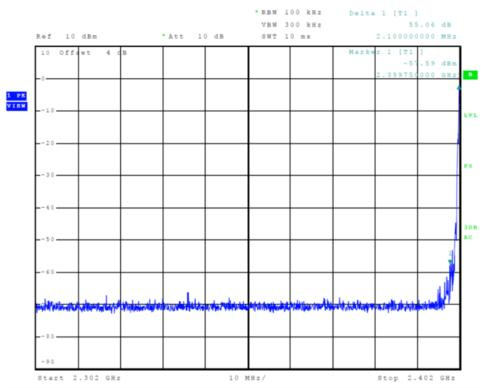
Figure 9 Plot of Transmitter Emissions (Low Band Edge, ANT GFSK)
