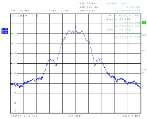
Figure 12 Plot of Transmitter Emissions (99% Occupied Bandwidth, BLE)
