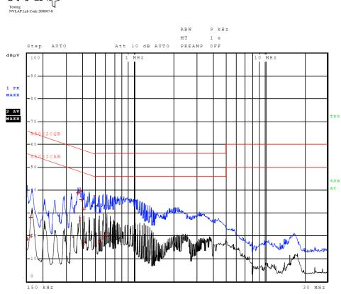
Figure 5 AC Line Conducted emissions of EUT line 1 (#4, EUT – 320-00072-02)
