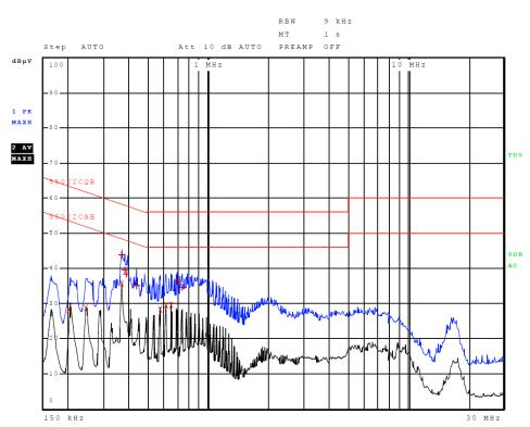
Figure 6 AC Line Conducted emissions of EUT line 2 (#4, EUT – 320-00072-02)
