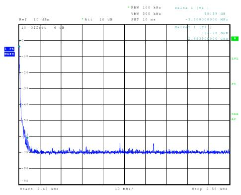
Figure 10 Plot of Transmitter Emissions (High Band Edge, ANT GFSK)
