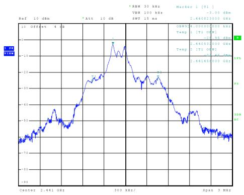
Figure 8 Plot of Transmitter Emissions (99% Occupied Bandwidth, ANT GFSK)
