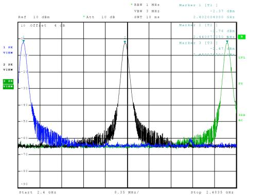
Figure 7 Plot of Transmitter Emissions (Operation in 2402-2480 MHz, ANT GFSK)
