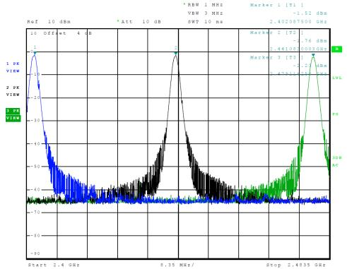
Figure 5 Plot of Transmitter Emissions (Operation in 2402-2479 MHz, ANT GFSK)
