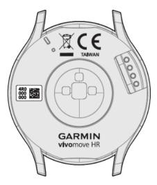
PMN is permanently molded into the back of the unit.
