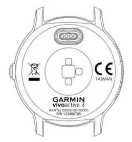
PMN is permanently affixed to the back of the unit via laser etching as shown above.
