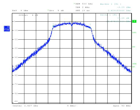
Figure 9 Plot of Transmitter 6-dB Occupied Bandwidth (802.11 g-mode)
