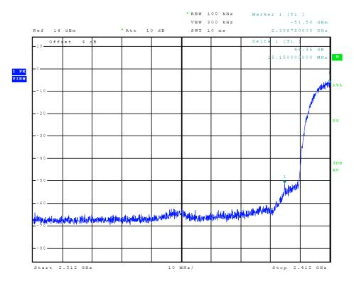
Figure 3 Plot of Lower Band Edge (802.11 b-mode)
