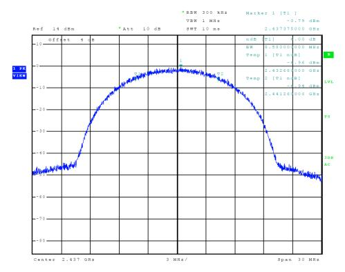
Figure 7 Plot of Transmitter 6-dB Occupied Bandwidth (802.11 b-mode)
