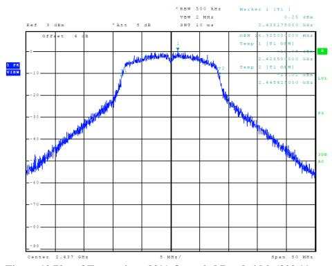
Figure 10 Plot of Transmitter 99% Occupied Bandwidth (802.11 g-mode)
