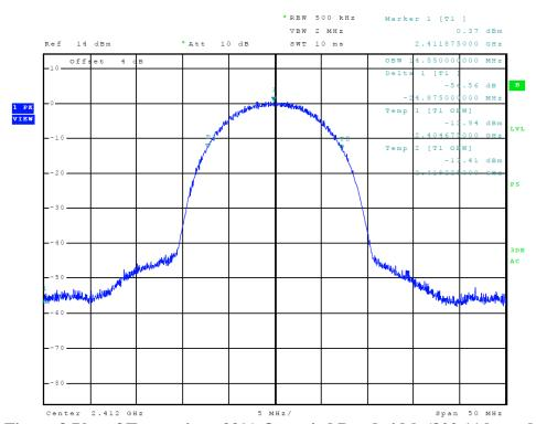
Figure 8 Plot of Transmitter 99% Occupied Bandwidth (802.11 b-mode)
