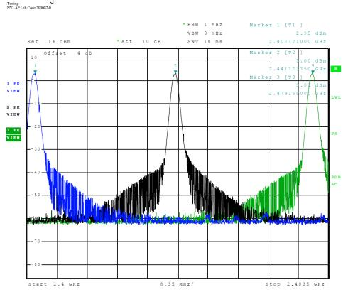
Figure 3 Plot of Transmitter Emissions (Operation in 2402-2479 MHz)
