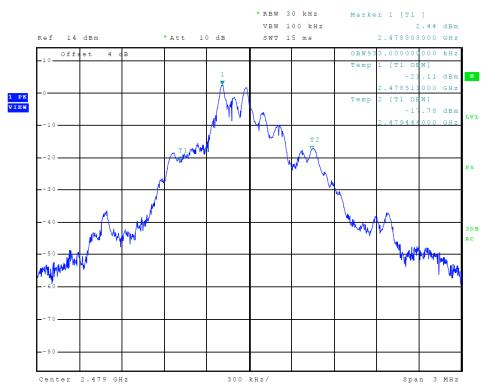
Figure 4 Plot of Transmitter Emissions (99% Occupied Bandwidth)
