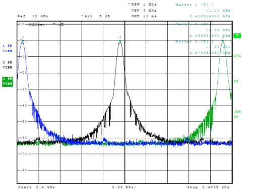
Figure 11 Plot of Transmitter Emissions (BLE 0x0F, Operation in 2402-2480 MHz)
