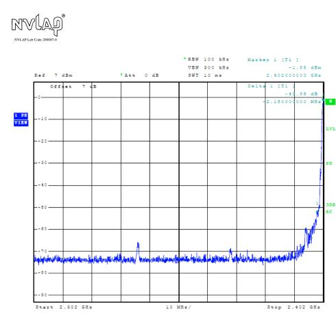
Figure 9 Plot of Transmitter Emissions (PRB29, Low Band Edge)
