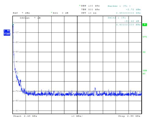
Figure 10 Plot of Transmitter Emissions (PRB29, High Band Edge)
