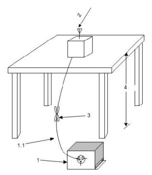
1—A LISN is optional for radiated measurements between 30 MHz and 1000 MHz but not allowed for measurements below 30 MHz and above 1000 MHz (see 6.3.1). If used, then connect EUT to one LISN. Unused LISN measuring port connectors shall be terminated in 50  $\Omega$  loads. The LISN may be placed on top of, or immediately beneath, the reference ground plane (see 6.2.2 and 6.2.3.2). 1.1—LISN spaced at least 80 cm from the nearest part of the EUT chassis.
