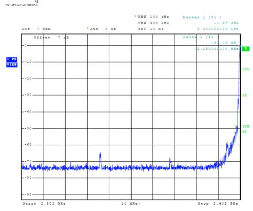
Figure 13 Plot of Transmitter Emissions (BLE 0x0F, PSK, Low Band Edge)
