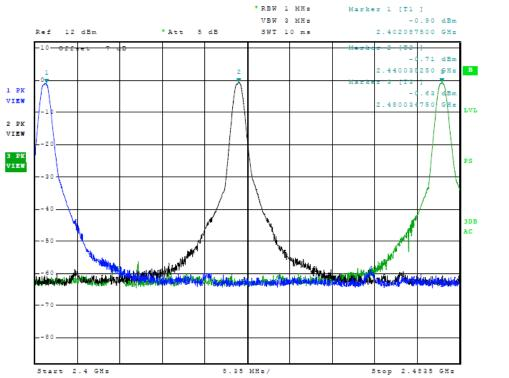
Figure 15 Plot of Transmitter Emissions (BLE 0x55, Operation in 2402-2480 MHz)
