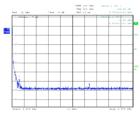
Figure 6 Plot of Transmitter Emissions (GFSK, High Band Edge)
