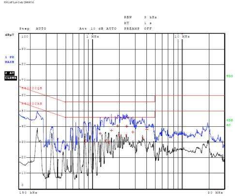
Figure 1 AC Line Conducted emissions of EUT line 1 (#4, EUT USB CPU Adapter)
