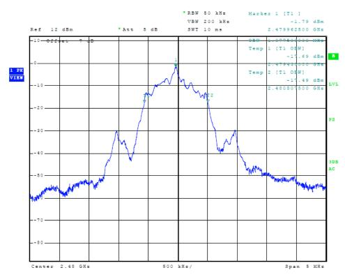
Figure 16 Plot of Transmitter Emissions (BLE 0x55, 99% Occupied Bandwidth)
