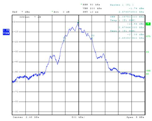
Figure 12 Plot of Transmitter Emissions (BLE 0x0F, 99% Occupied Bandwidth)
