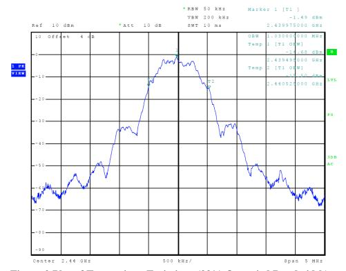
Figure 2 Plot of Transmitter Emissions (99% Occupied Bandwidth)
