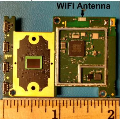
Sensor board with camera and shield
