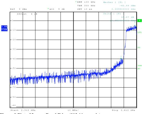
Figure 8 Plot of Lower Band Edge (802.11 g-mode)
