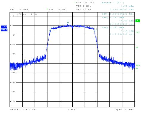
Figure 20 Plot of Transmitter 99% Occupied Bandwidth (802.11 n-mode)
