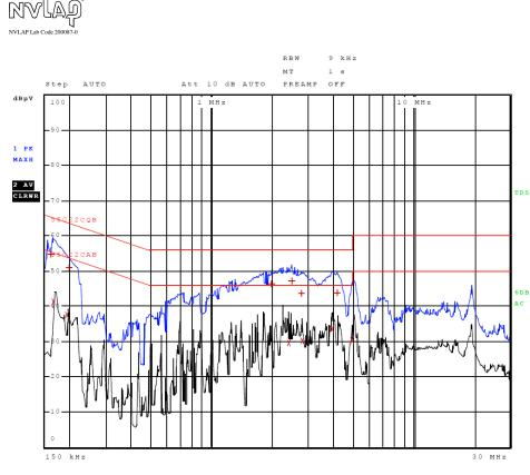
Figure 1 AC Line Conducted emissions of EUT line 1 (#2, EUT - CPU)
