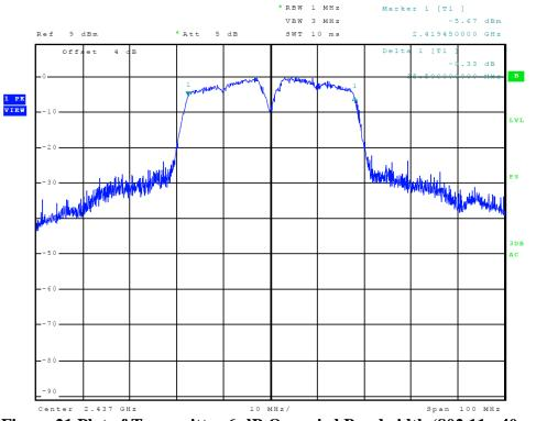
Figure 21 Plot of Transmitter 6-dB Occupied Bandwidth (802.11 n40-mode)
