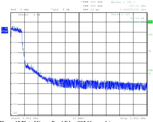
Figure 12 Plot of Upper Band Edge (802.11 g-mode)
