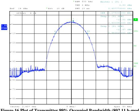
Figure 16 Plot of Transmitter 99% Occupied Bandwidth (802.11 b-mode)
