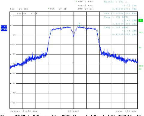
Figure 22 Plot of Transmitter 99% Occupied Bandwidth (802.11 n40-mode)
