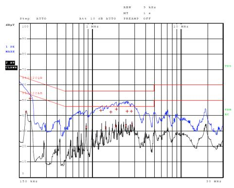
Figure 2 AC Line Conducted emissions of EUT line 2 (#2, EUT - CPU)
