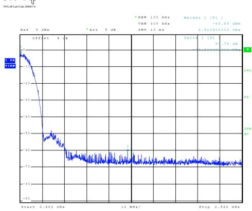
Figure 11 Plot of Upper Band Edge (802.11 b-mode)
