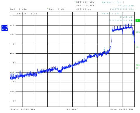
Figure 10 Plot of Lower Band Edge (802.11 n40-mode)
