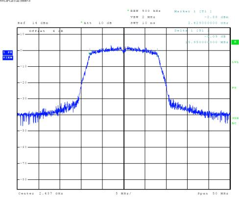
Figure 17 Plot of Transmitter 6-dB Occupied Bandwidth (802.11 g-mode)
