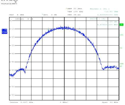
Figure 15 Plot of Transmitter 6-dB Occupied Bandwidth (802.11 b-mode)
