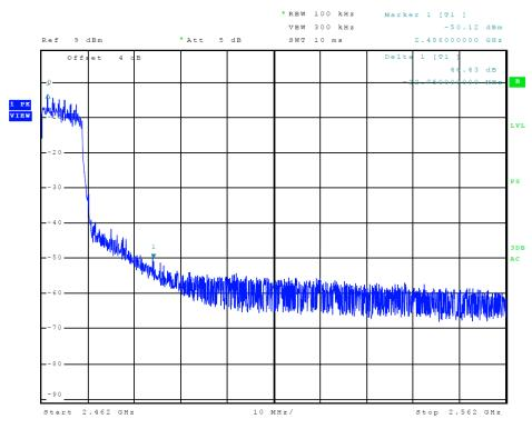
Figure 13 Plot of Upper Band Edge (802.11 n-mode)
