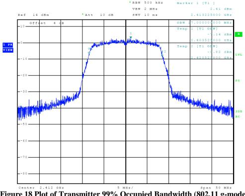
Figure 18 Plot of Transmitter 99% Occupied Bandwidth (802.11 g-mode)
