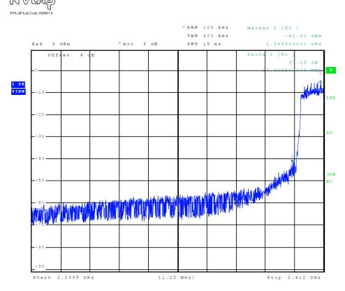
Figure 9 Plot of Lower Band Edge (802.11 n-mode)
