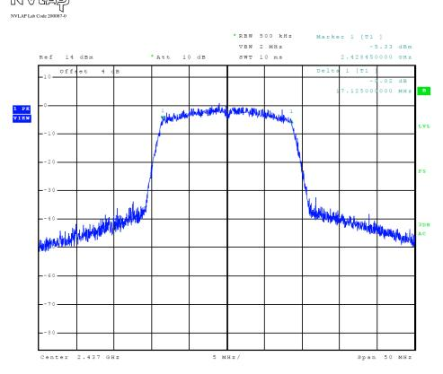
Figure 19 Plot of Transmitter 6-dB Occupied Bandwidth (802.11 n-mode)
