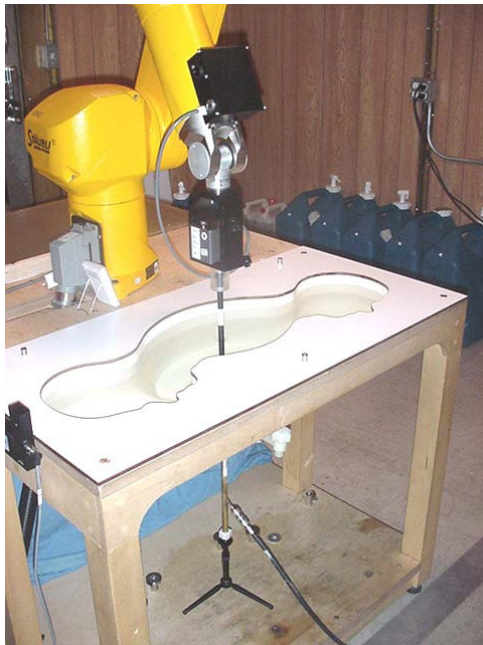
DASY 4 SAR System with SAM Phantom
