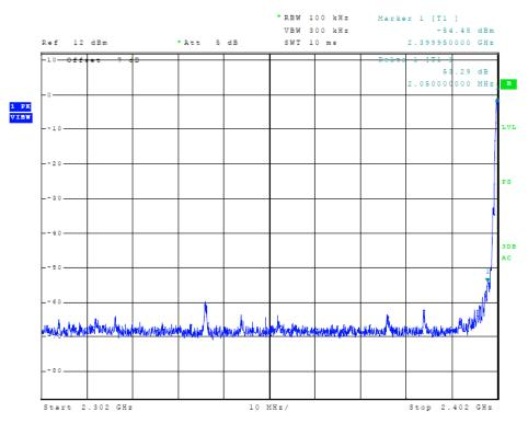
Figure 15 Plot of Transmitter Emissions (Low Band Edge, BLE 0x0F)
