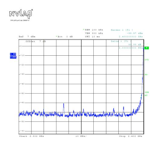
Figure 11 Plot of Transmitter Emissions (Low Band Edge, PRB29)
