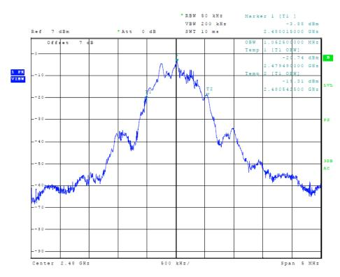
Figure 10 Plot of Transmitter Emissions (99% Occupied Bandwidth, PRB29)
