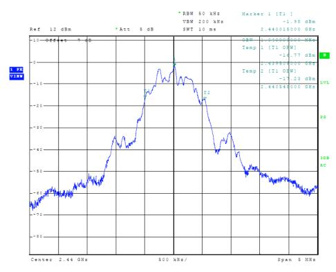
Figure 14 Plot of Transmitter Emissions (99% Occupied Bandwidth, BLE 0x0F)
