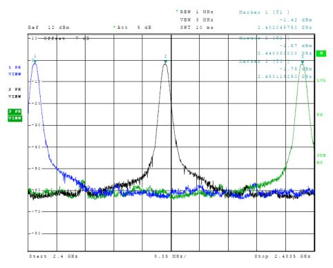
Figure 9 Plot of Transmitter Emissions (Operation in 2402-2480 MHz, PRB29)
