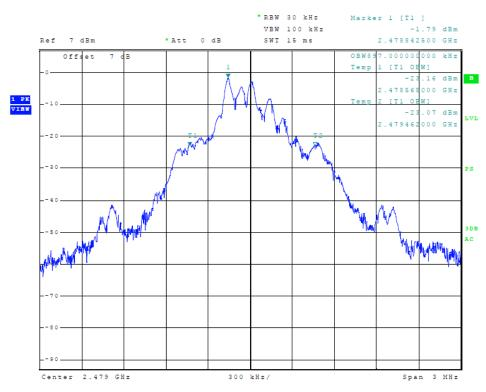
Figure 6 Plot of Transmitter Emissions (99% Occupied Bandwidth, GFSK)
