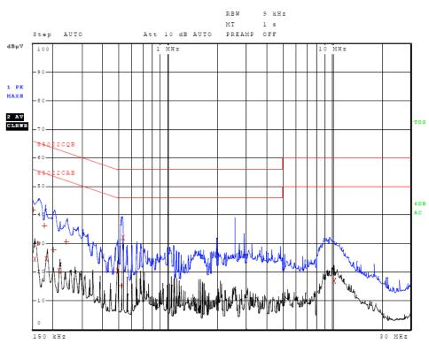
Figure 2 AC Line Conducted emissions of EUT line 2 (#3, EUT – AC Adapter)
