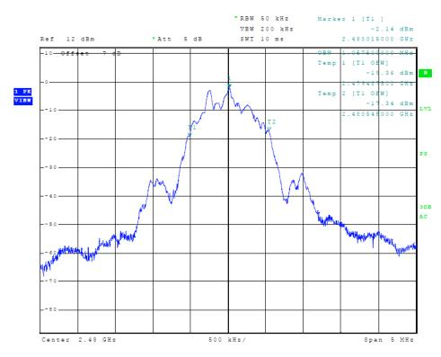
Figure 18 Plot of Transmitter Emissions (99% Occupied Bandwidth, BLE 0x55)
