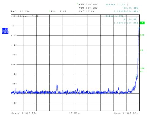
Figure 19 Plot of Transmitter Emissions (Low Band Edge, BLE 0x55)
