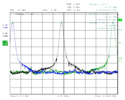
Figure 13 Plot of Transmitter Emissions (Operation in 2402-2480 MHz, BLE 0x0F)
