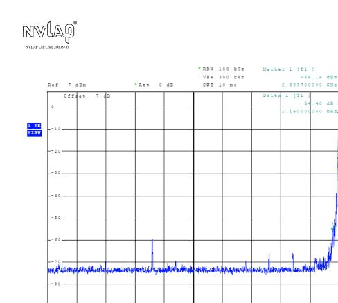
Figure 7 Plot of Transmitter Emissions (Low Band Edge, GFSK)
