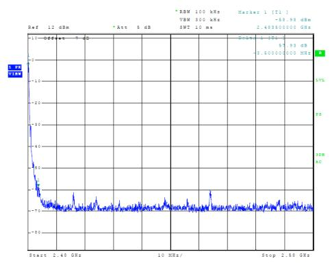
Figure 16 Plot of Transmitter Emissions (High Band Edge, BLE 0x0F)
