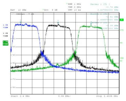
Figure 9 Plot of Transmitter Emissions in Operational Frequency (802.11 n-Mode)
