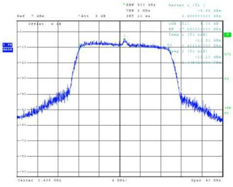
Figure 20 Plot of Transmitter 6-dB Occupied Bandwidth (802.11 n-mode)
