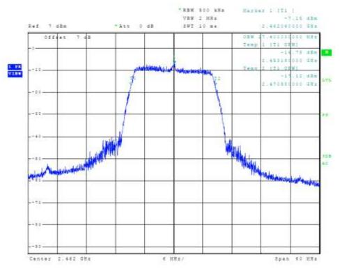
Figure 19 Plot of Transmitter 99% Occupied Bandwidth (802.11 g-mode)
