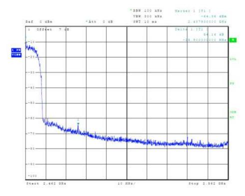
Figure 13 Plot of Upper Band Edge (802.11 b-mode)
