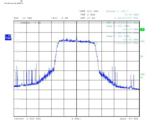
Figure 21 Plot of Transmitter 99% Occupied Bandwidth (802.11 n-mode)
