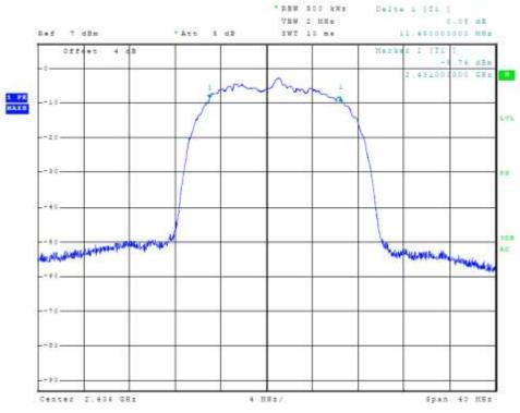
Figure 16 Plot of Transmitter 6-dB Occupied Bandwidth (802.11 b-mode)
