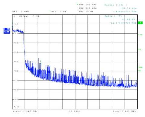
Figure 15 Plot of Upper Band Edge (802.11 n-mode)
