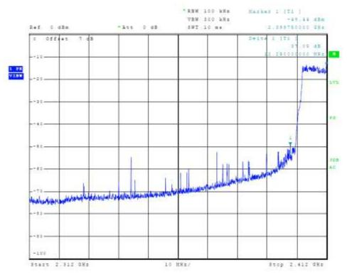
Figure 11 Plot of Lower Band Edge (802.11 g-mode)
