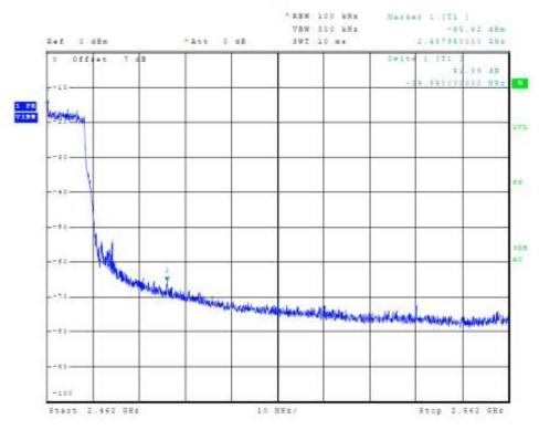
Figure 14 Plot of Upper Band Edge (802.11 g-mode)
