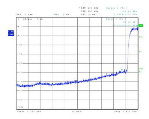
Figure 10 Plot of Lower Band Edge (802.11 b-mode)
