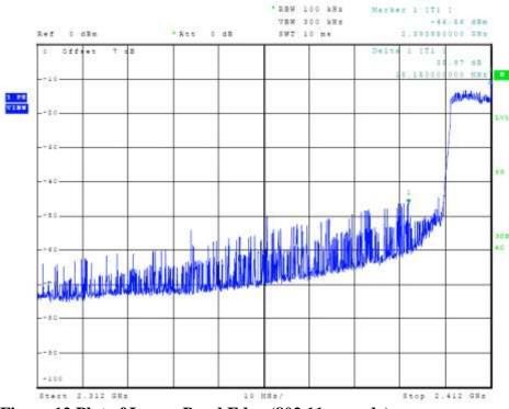
Figure 12 Plot of Lower Band Edge (802.11 n-mode)
