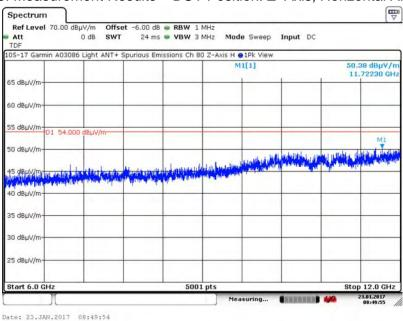
A.19.6. Measurement Results – DUT Position: Z-Axis, Vertical Antenna
