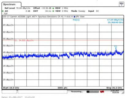
A.14.4. Measurement Results - DUT Position: Y-Axis, Vertical Antenna
