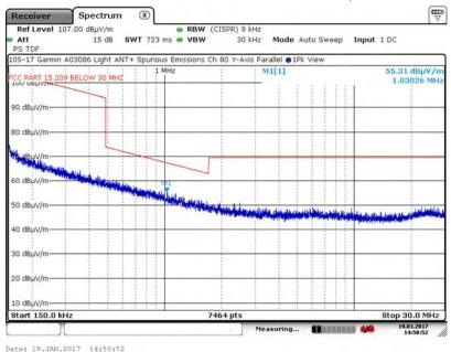
A.16.4. Measurement Results - DUT Position: Y-Axis, Perpendicular Antenna
