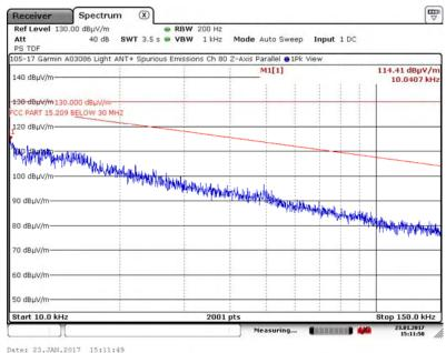
A.15.6. Measurement Results - DUT Position: Z-Axis, Perpendicular Antenna
