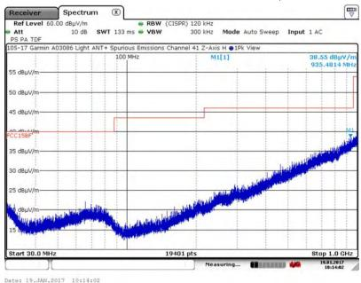
A.10.6. Measurement Results - DUT Position: Z-Axis, Vertical Antenna
