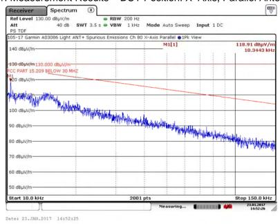
A.15.1.2. Measurement Results - DUT Position: X-Axis, Perpendicular Antenna
