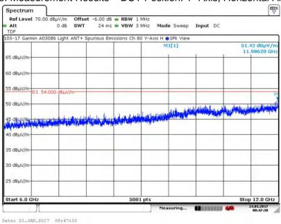
A.19.4. Measurement Results – DUT Position: Y-Axis, Vertical Antenna
