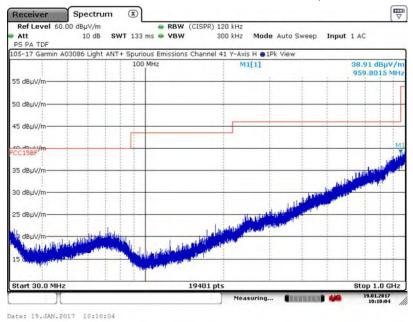
A.10.4. Measurement Results - DUT Position: Y-Axis, Vertical Antenna
