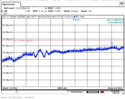
A.18.4. Measurement Results - DUT Position: Y-Axis, Vertical Antenna
