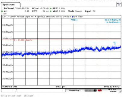
A.12.6. Measurement Results - DUT Position: Z-Axis, Vertical Antenna
