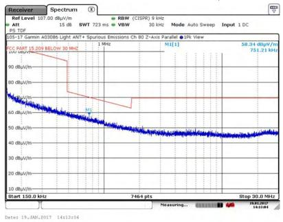
A.16.6. Measurement Results – DUT Position: Z-Axis, Perpendicular Antenna
