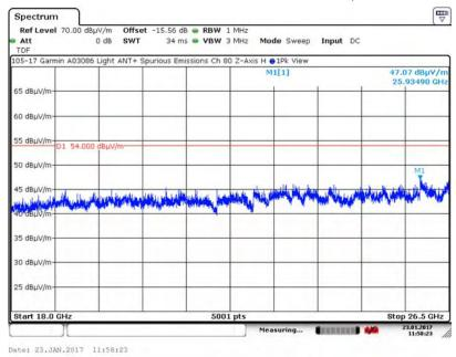
A.21.6. Measurement Results - DUT Position: Z-Axis, Vertical Antenna
