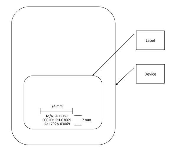
Back of device (Label Placed Inside battery compartment not on battery door)
